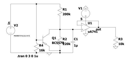
This circuit uses time-delayed RC circuit to delay the command received from the switch. This will give enough time for the controller to switch its directions safely without interruption.
