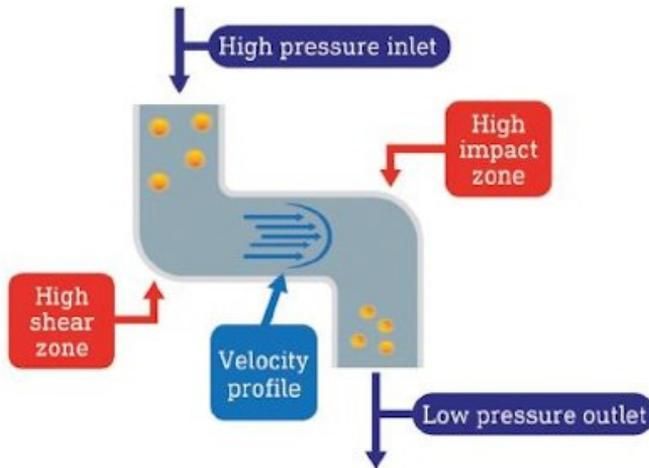
**Figure 1. Schematic representation of the phenomenon happening in the interaction chamber of HPH**
