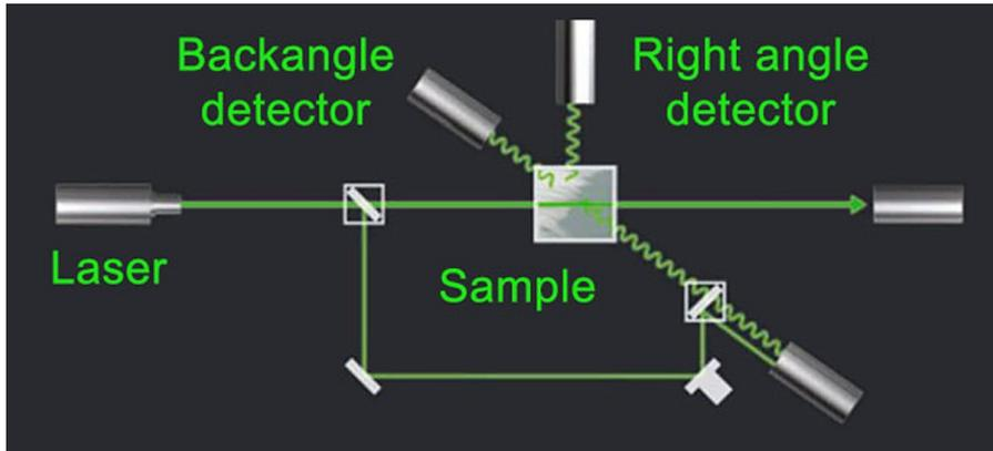
Light from the laser light source illuminates the sample in the cell. The scattered light signal is collected with one of two detectors, either at a 90 degree (right angle) or 173 degree (back angle) scattering angle. The provision of both detectors allows more flexibility in choosing measurement conditions. Particles can be dispersed in a variety of liquids. Only liquid refractive index and viscosity needs to be known for interpreting the measurement results.
