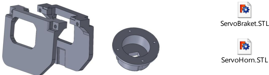
Figure 18-5 – Retrofit 3D Model
