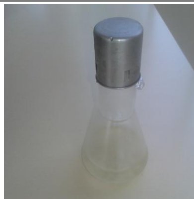
the change of smell shows that ethyl acetate is formed Of 30ml acetic acid +30ml ethanol+17ml sulfuric acid we got 15 ml ethyl acetate
