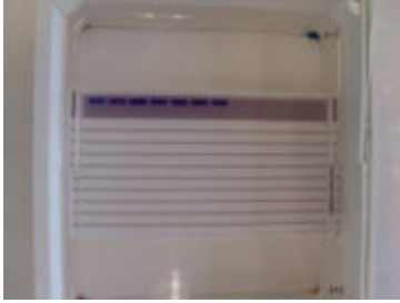
Agarose gel with samples loaded in the slots, before the electrophoresis process
