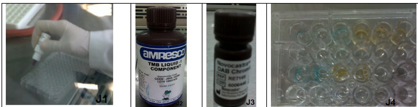
Figure 30: add drop of the Novolink polymer in each well as J1) then add in part of wells TMB (J2) and in the second part DAB (J3), J4) observe the wells that have TMB change it color to blue after many seconds.
