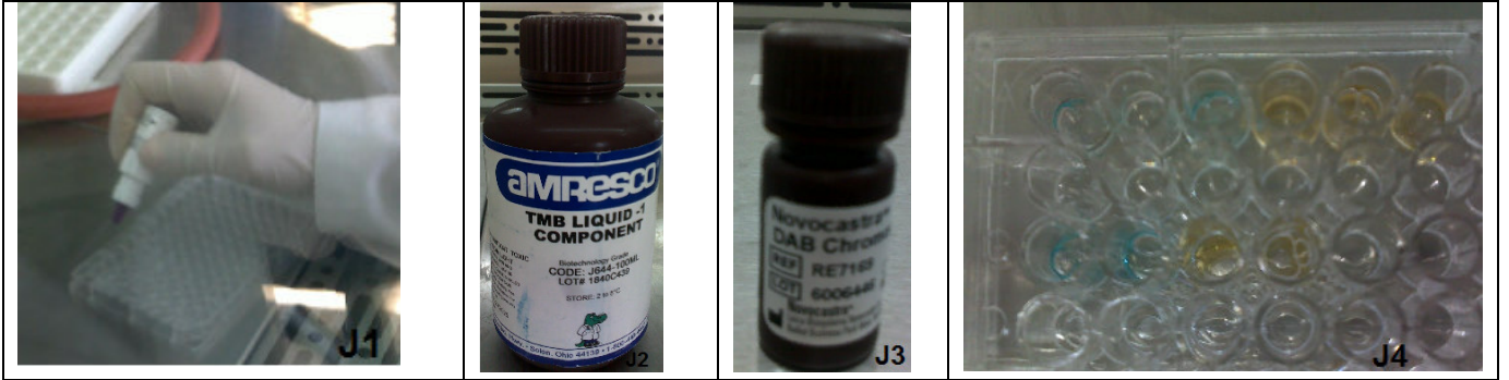
Figure 30: add drop of the Novolink polymer in each well as J1) then add in part of wells TMB (J2) and in the second part DAB (J3), J4) observe the wells that have TMB change it color to blue after many seconds.
