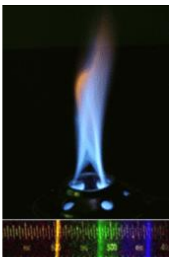
Ethanol burning with its spectrum depicted
