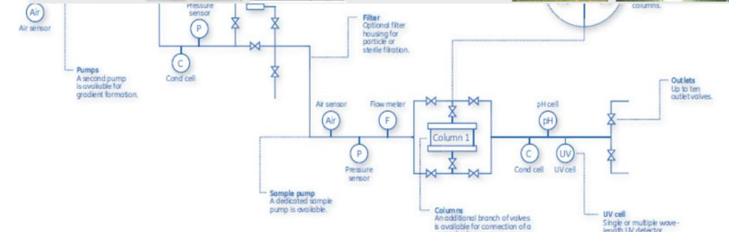
Fig 2. The liquid flow path.
