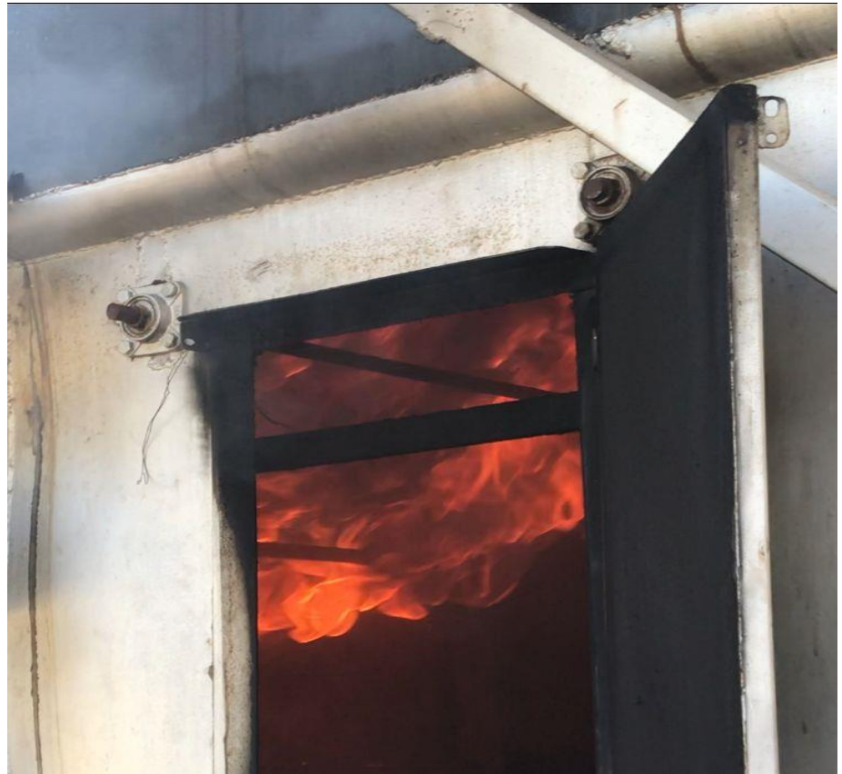
Stage9: Test 3 expansion valve to the ambient
