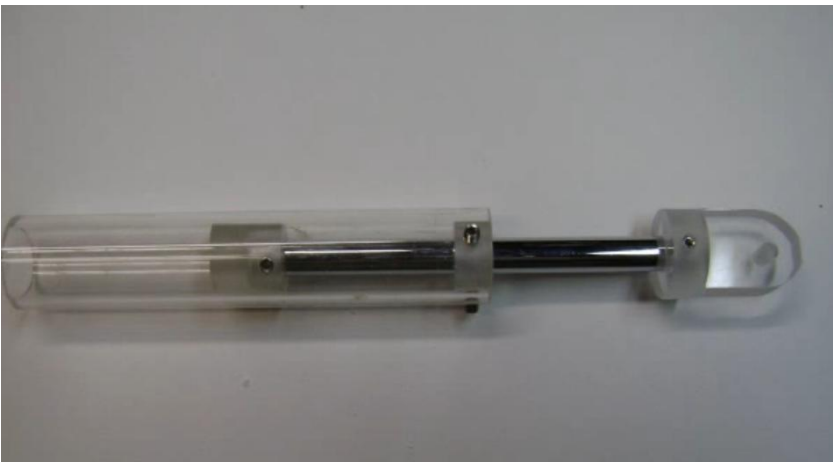
Plunger tab assembled and test fit
