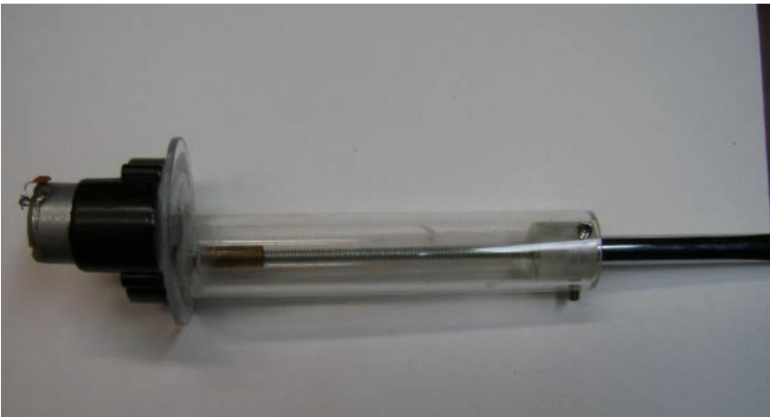
Main housing tube attached to motor plate and plunger threaded on rod
