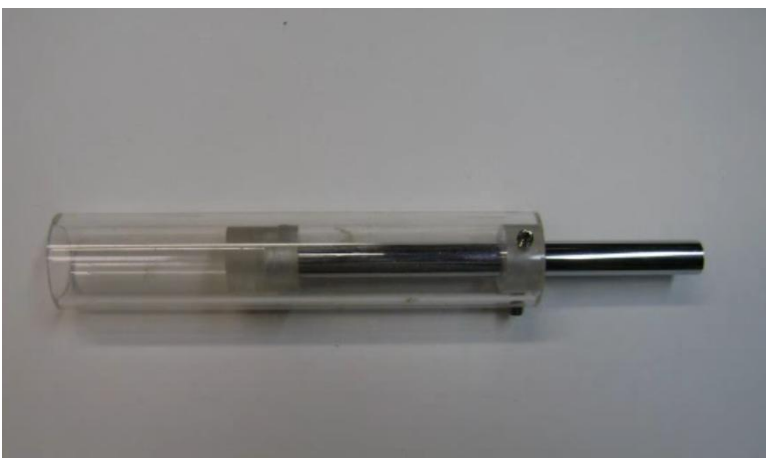
Plunger assembly test fit into tube with centering ring set screwed into place
