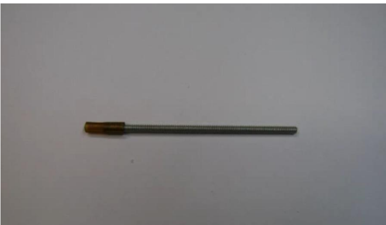
Threaded rod and tubing coupler
