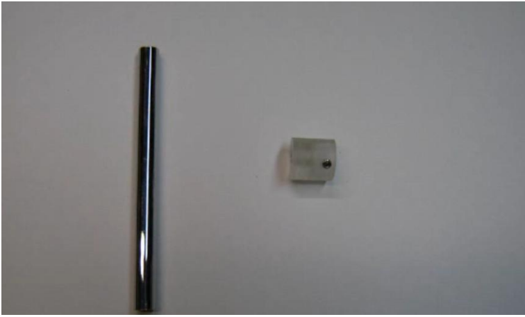
Brass tube-3/8 O.D and a plastic nut to fit and secure with setscrews
