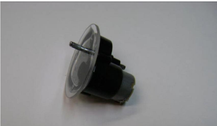
Motor shaft needs to be 90-degree angle on plate
