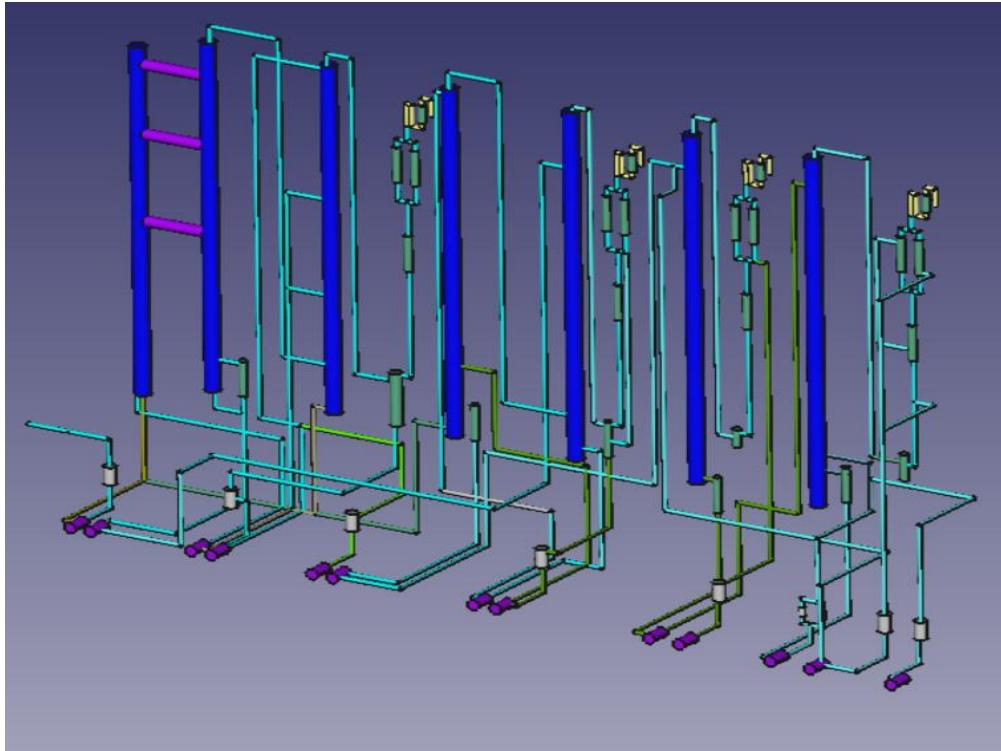
is an ongoing separation process in which a liquid mixture of two or more miscible components is continuously fed into the process and physically separated into two or more products by preferentially boiling the more volatile (i.e., lower boiling point) components out of the mixture.
