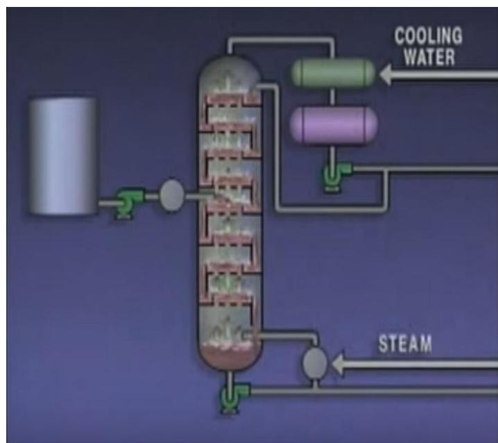
Industrial distillation is typically performed in large, vertical cylindrical columns (see the adjacent photographs) commonly referred to as *distillation columns*, *distillation towers* or *fractionators* with diameters ranging from **about 65 centimeters to 11 meters** and heights ranging from about 6 meters to 60 meters or more.
