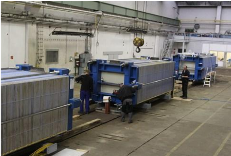
Figure 4: Three units of 2 MW Enertrag alkaline electrolyser unit - 1000 m 3 / h
