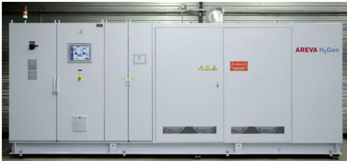
Figure 17: Electrolyser PEM AREVA H 2 GEN/CETH 2 120 Nm 3 /h (2015)
