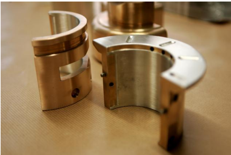
Figure 16: Min bearings for steam turbine
