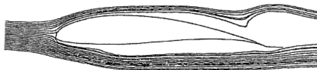
Fig. 7.26 Instantaneous streamlines over Wortmann airfoil (FX63-137)—laminar flow (unsteady results) ( Re = 100000 , M = 0.5 , \text{Alpha} = 0.0 \text{ deg.} ) Non-dimensional time T_n = 7.04
