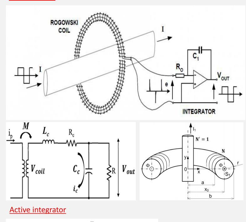
The Rogowski coil is defined as an electrical device that is used to measure alternating current (AC).
