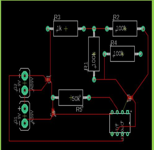
Using the schematic on Eagle CAD, we build the active integrator which is connected to the coil.
