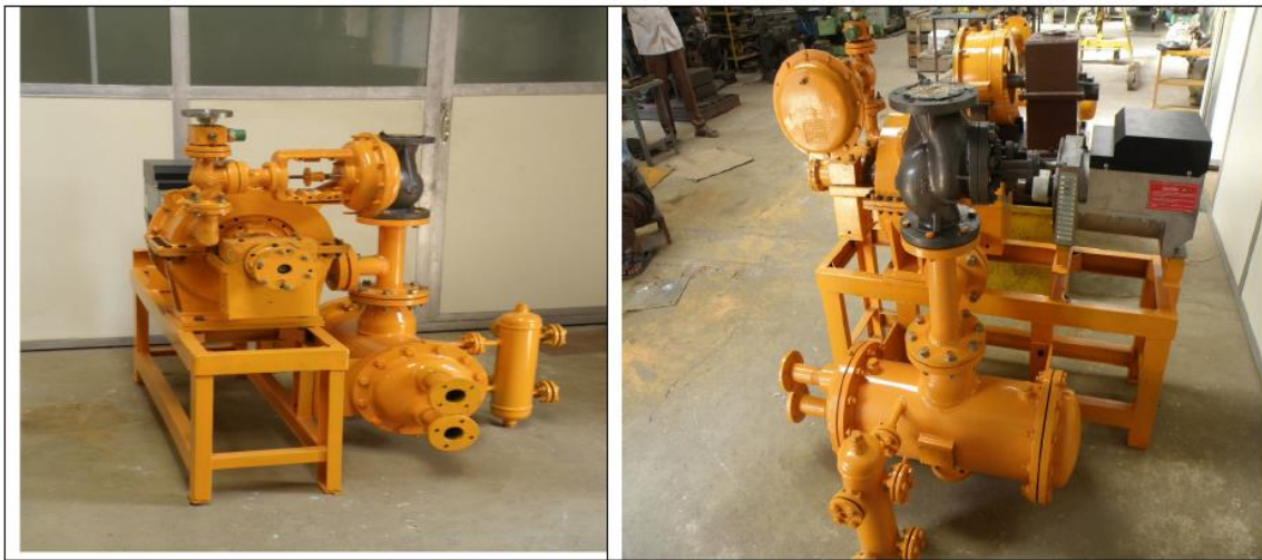
Left – 10 KW Unit specially mounted on a Frame (on request) with Water Cooled Condenser at side.
