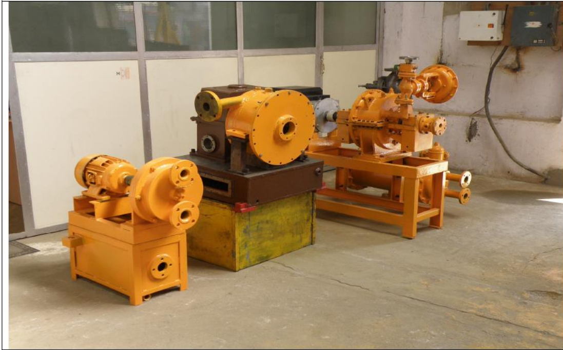
L to R = 5 KW CHP Unit, 30 KW Integral with Gear Box and 10 KW Unit on a Frame with Water Cooled Condenser.
