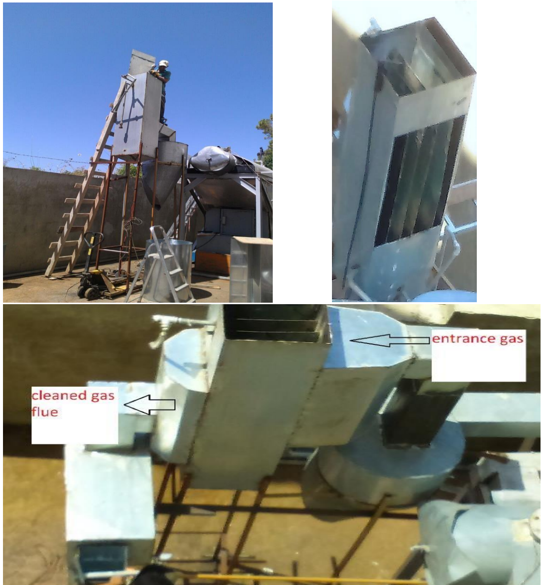
Figure 39: insert of plate (iron) & copper wire.
