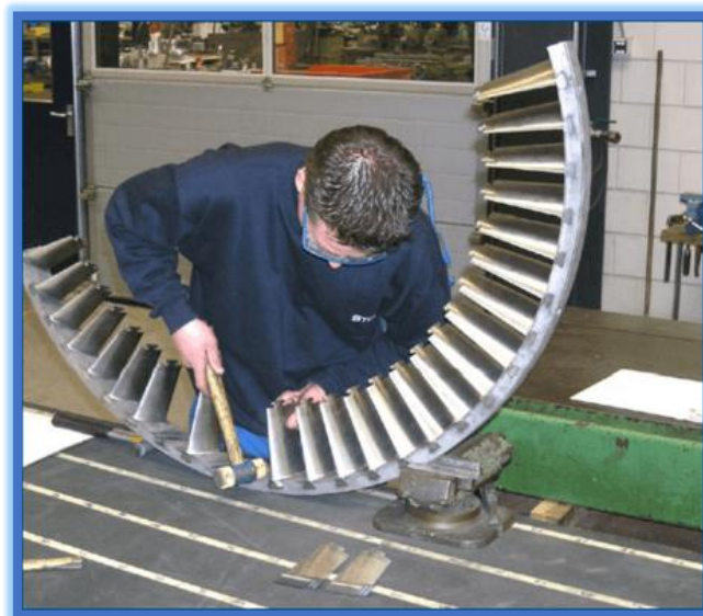
Figure 14: method of putting fixed blade
