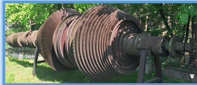
Figure I-12: Parsons Turbine from the Polish destroyer ORP Wicher .
