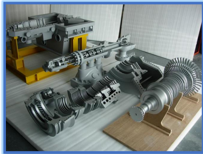
Figure 16: steam turbine model- inner parts
