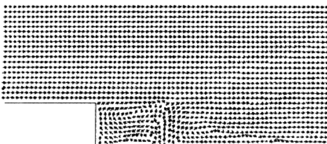
Fig. 7.17 Velocity vectors with H_2 injection
