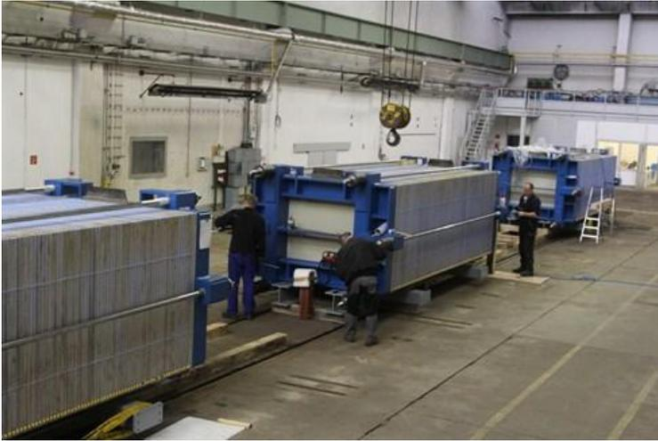
Figure 4: Three units of 2 MW Enertrag alkaline electrolyser unit - 1000 m<sup>3</sup> / h
