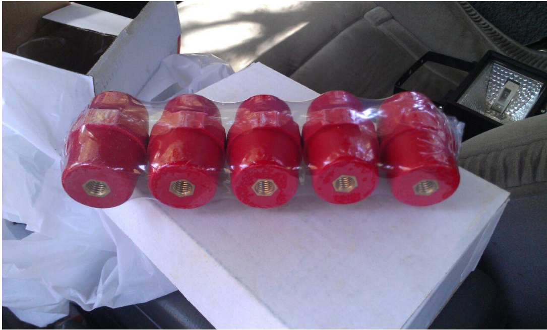
Figure 35: insulator used to ESP in the power plant.
