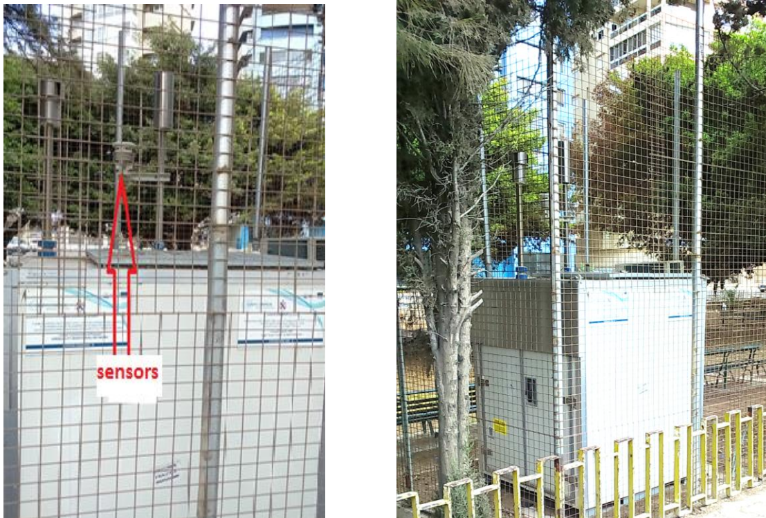
Figure 69: System to analyzer the concentration of gas in air of Tripoli
