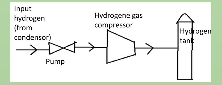
Connect the Hydrogen source to the diaphragm compressor inlet using a tapped hose, and leave the tap closed to prevent the gas from flowing. Use an external pump to push the gas into the compressor since the compressor itself sucks the gas from the inlet into its hydraulic pump. Make sure that the connection between the Hydrogen source and the compressor is air tight.
