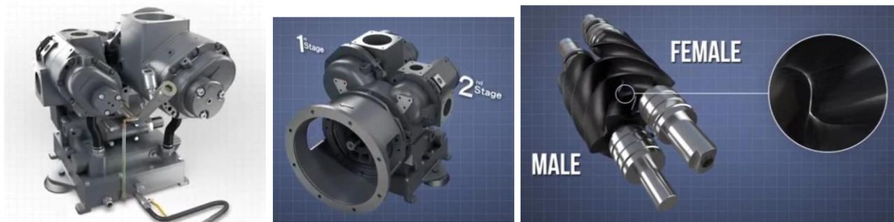
The oil-free industrial air compressor is a two-stage oil-free compressor unit. both compression stages comprise male and female rotors, with special protective coating. there's no physical contact either between the matched rotor pairs or the rotors and the air and casing. everything is separated by a precisely engineered air gap. The male rotors of both the first and second stages are driven by a single main gear at the back of the air end.
