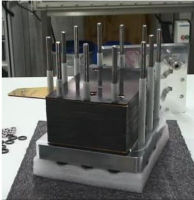
**Fig. 73: Remove the end plate from the stack**
