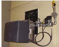
Natural gas burner equipping an industrial cooking oven
