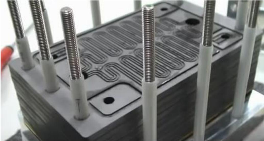
**Fig. 75: First cell next to the current collector**
