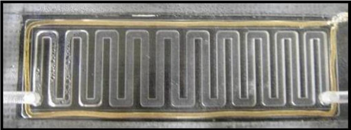
*Fig. 67: Condensation of water produced by a PEMFC on the air channel wall. The gold wire around the cell ensures the collection of electric current*
