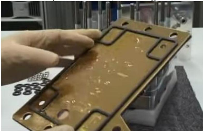
**Fig. 74: Remove the current plate collector, with the gasket from the stack**
