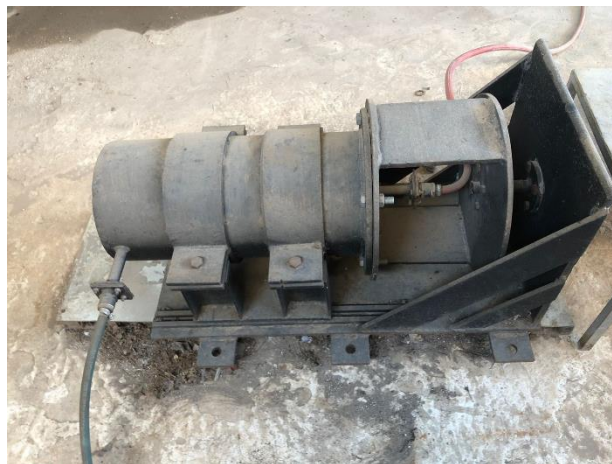
Figure 2-2. Fuel Burner Plant
