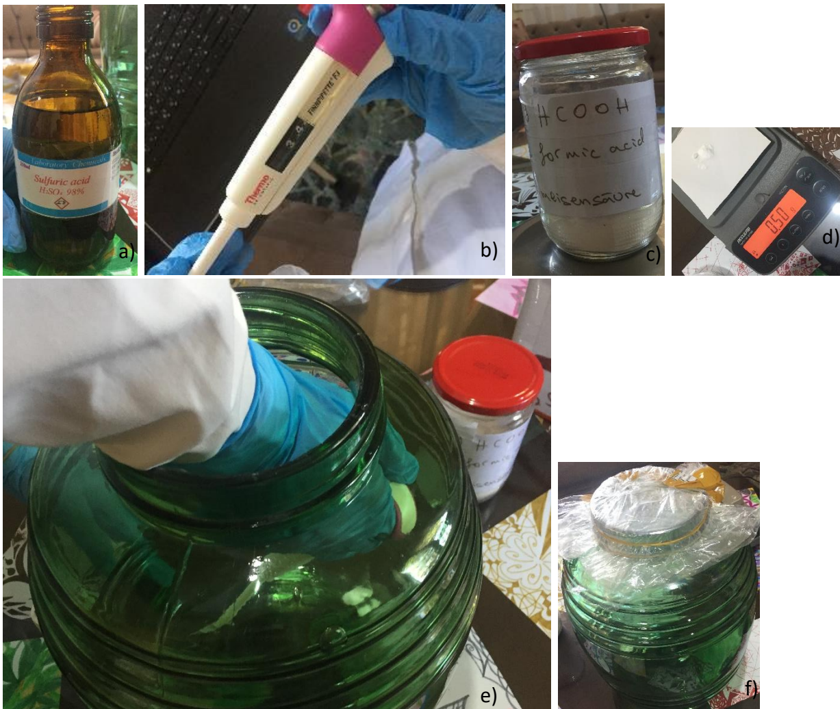
Figure 13 a) sulfuric acid b) micropipette c) formic acid d) balance e) putting them in the volume f) hermetic closure of container
