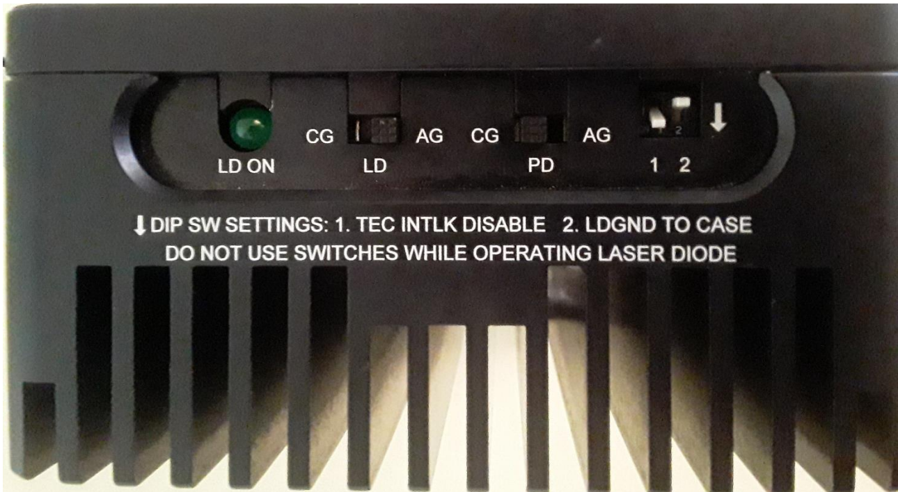
Figure 9 CC mode, the LD is anode grounded and the PD is cathode grounded
