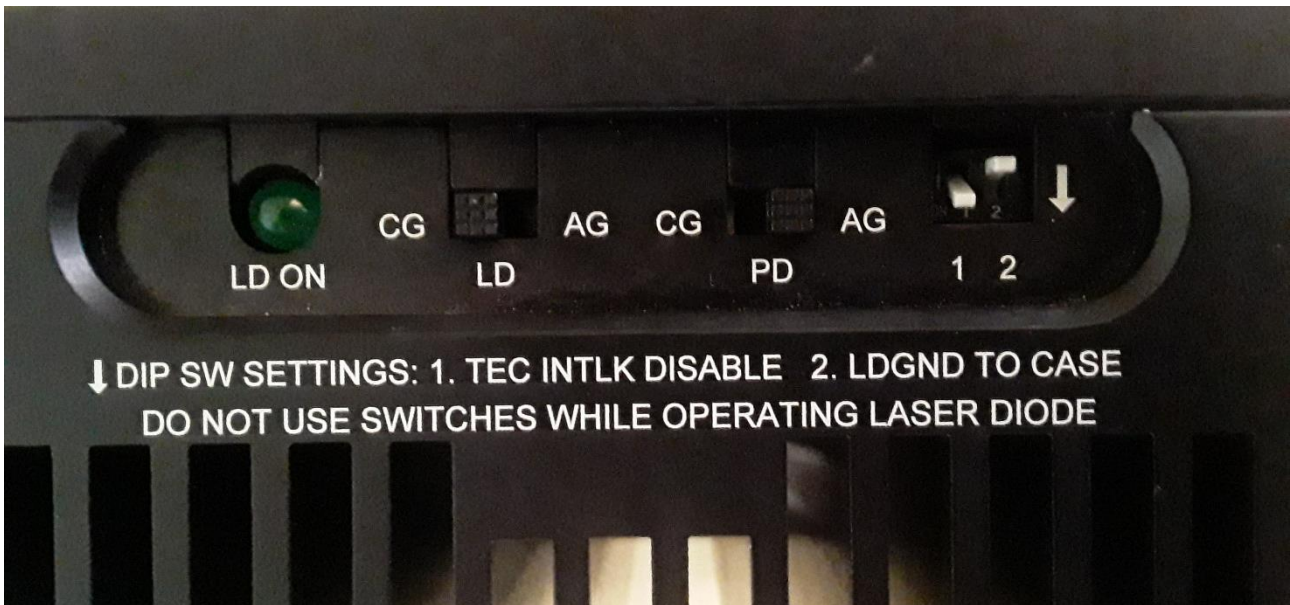
Figure 8 the CP mode, LD is cathode grounded and the PD is anode grounded
