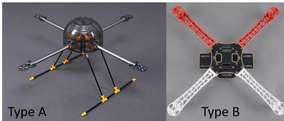
Figure 3.7. Quadcopter frames chosen for the project
