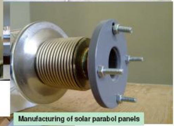
Solar vacuum pipe
