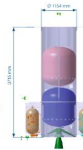
Bi-propellant UPS B3 Propellant Loading Mass: 2441 kg
