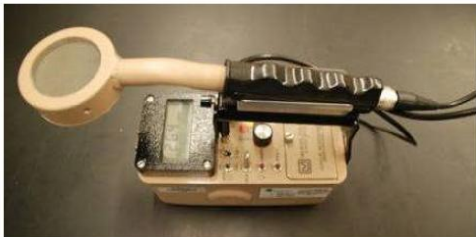
Figure 35 Portable contamination meter with pancake probe
