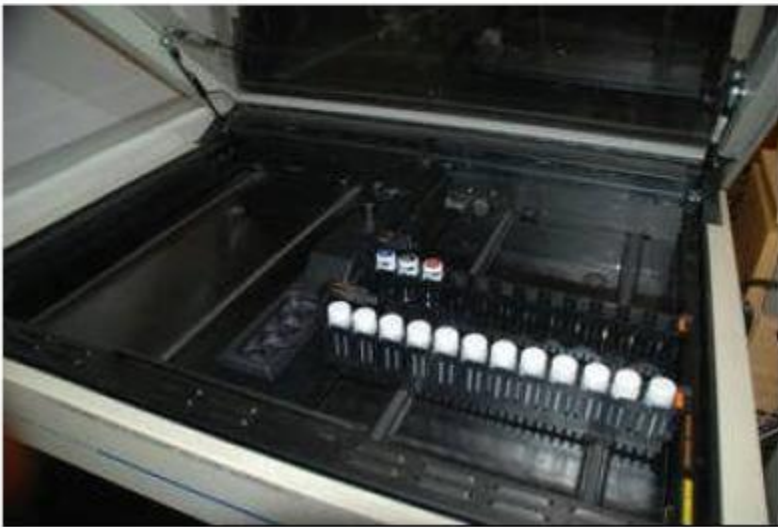
Figure 44 Commercial LSC counter (top) and detail of trays with vials (bottom)
