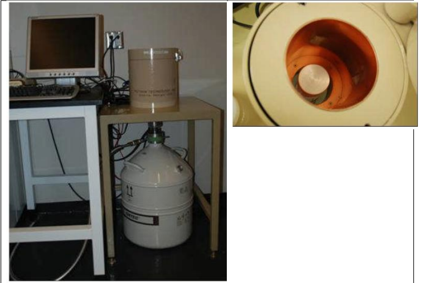
Figure 34 Commercial HPGe system (left) and detail of lead castle (right)
