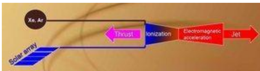
Figure 3.14: Hall Effect propulsion
