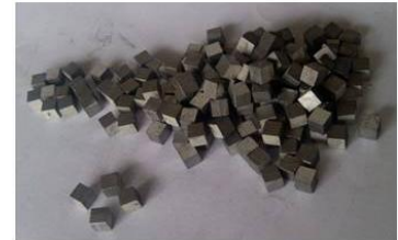
Thermoelectric materials on the basis of bismuth telluride Bi_2Te_3
