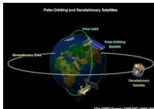
Figure 1.5: Third law of Kepler (satellite polar orbiting is faster than geostationary orbiting because of radius)
