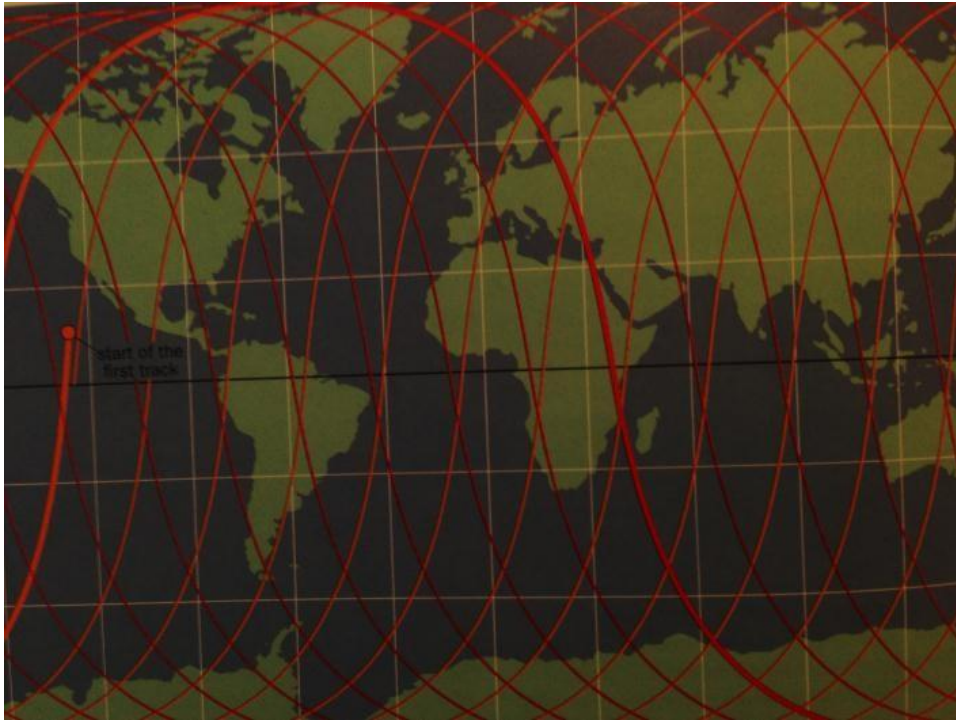
Figure 2.5: All rotations of the satellite around the earth during the day
