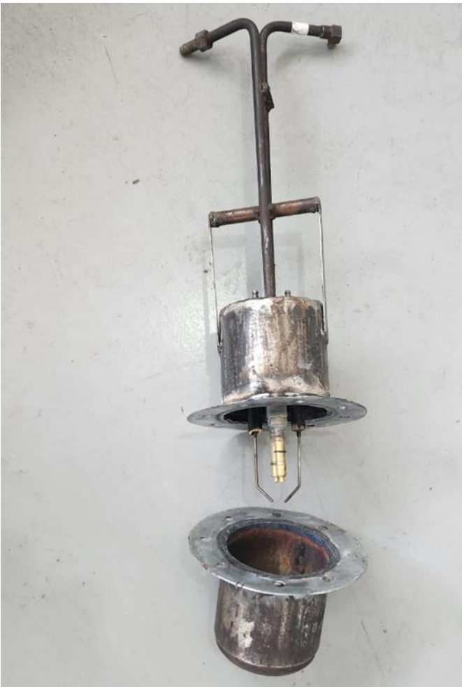
Picture 9: Fuel and oxidizer inlet to combustion chamber
