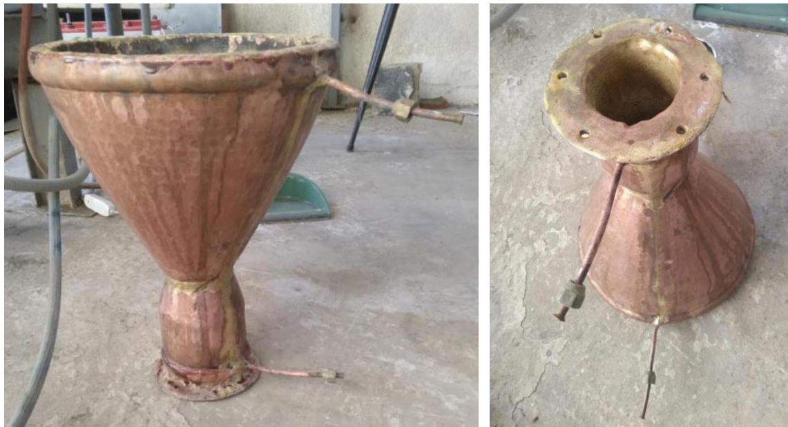
Figure 13.28 Thrust Chamber After Integration of Propellant Inlets and Outlets for Regenerative Cooling
