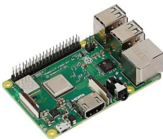
Figure 2-41 Raspberry Pi picture
