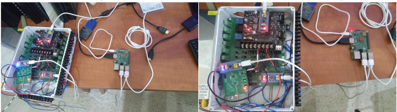
Picture 15: Connected the Raspberry with ACS Board, Transvers Board, Power Charge Board.
