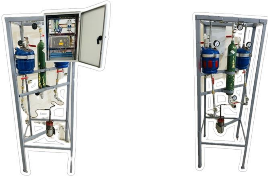
Picture 1: Testrig For Satellite Propulsion
