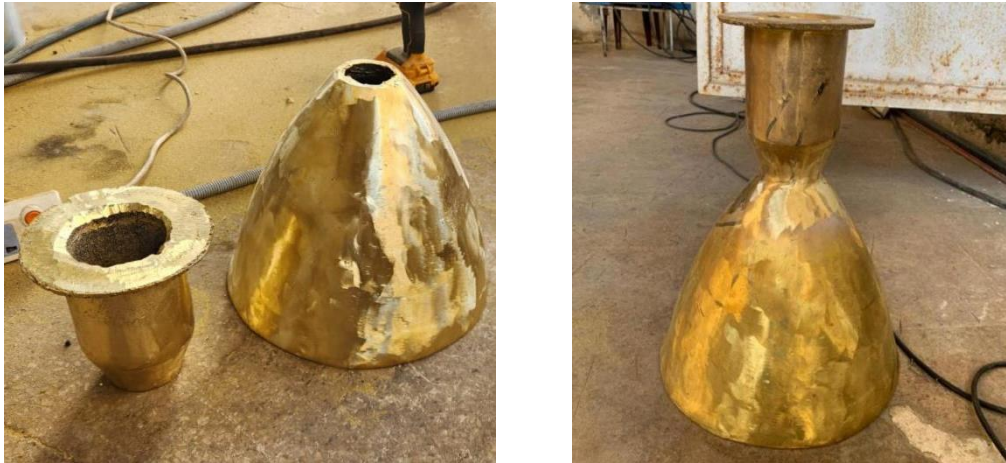
Figure 13.24 Copper-Formed Combustion Chamber and Nozzle Fabricated at AECENAR
