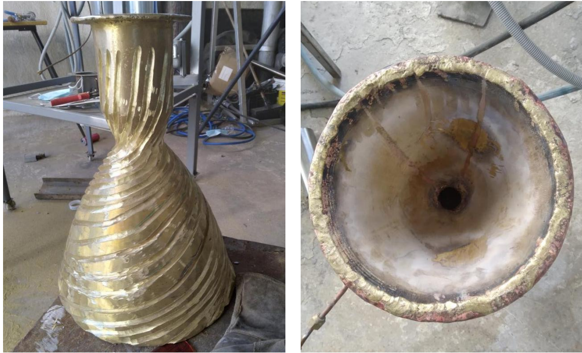
Figure 13.27 Realization of Pipes Layout for Regenerative Cooling
