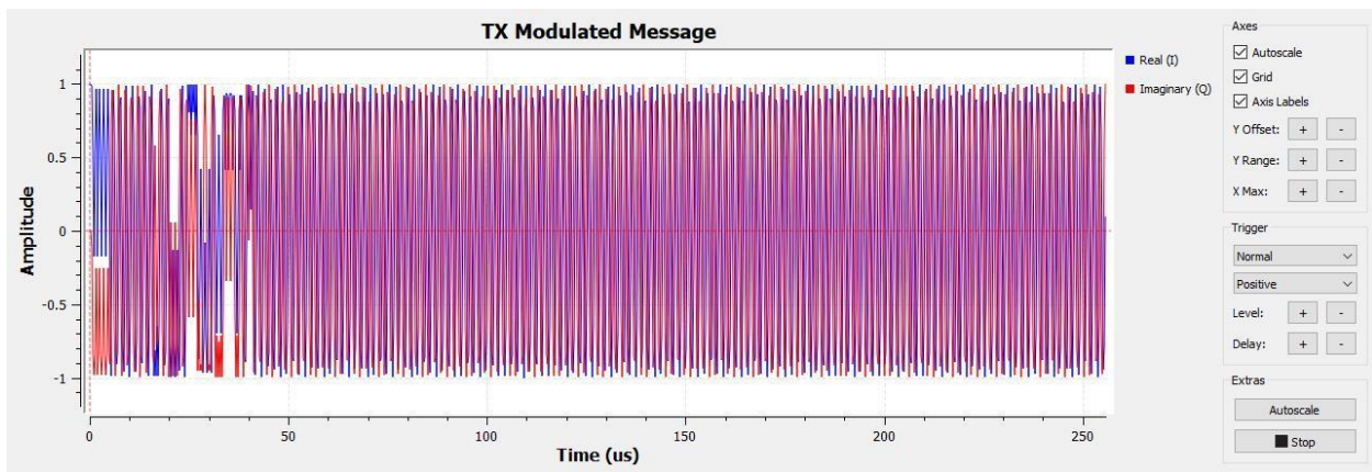
Figure 8-13 GFSK modulation block output
