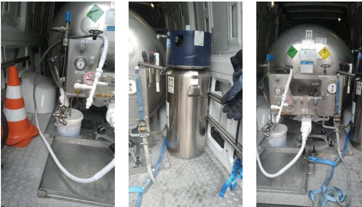
Figure 13.26 Oxidizer Tank Designed for 45 Liters of LOX, Photographed in Germany
