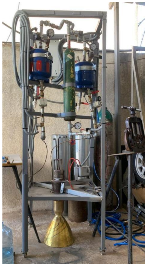
Figure 13.25 Integration of the Copper Thrust Chamber into the Orbit Change Test Stand at AECENAR
