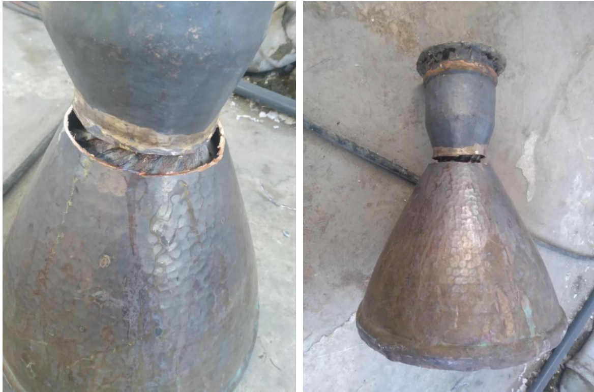
Figure 13.29 Integration of the Closeout Wall into the Regenerative Cooling System at AECENAR
