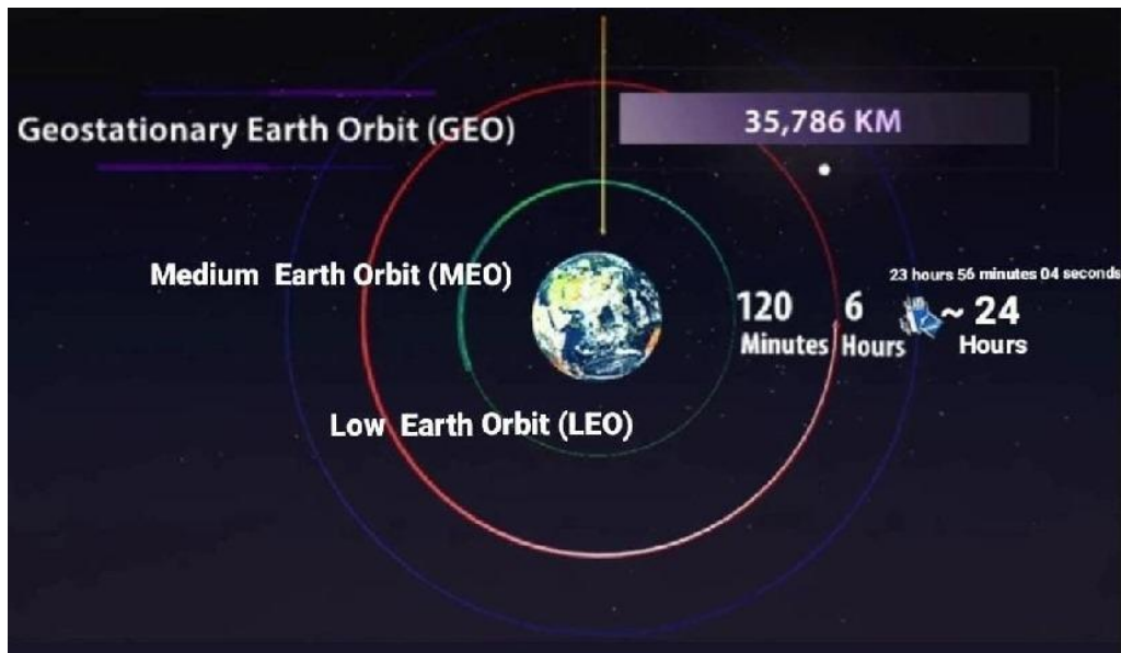
Figure 13.1 illustration of Orbital Altitudes: Low Earth Orbit (LEO), Medium Earth Orbit (MEO), and Geostationary Earth Orbit (GEO)
