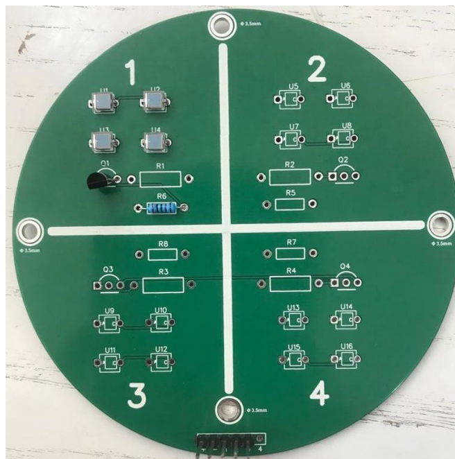
Figure 2-8 Sun sensor PCB board
