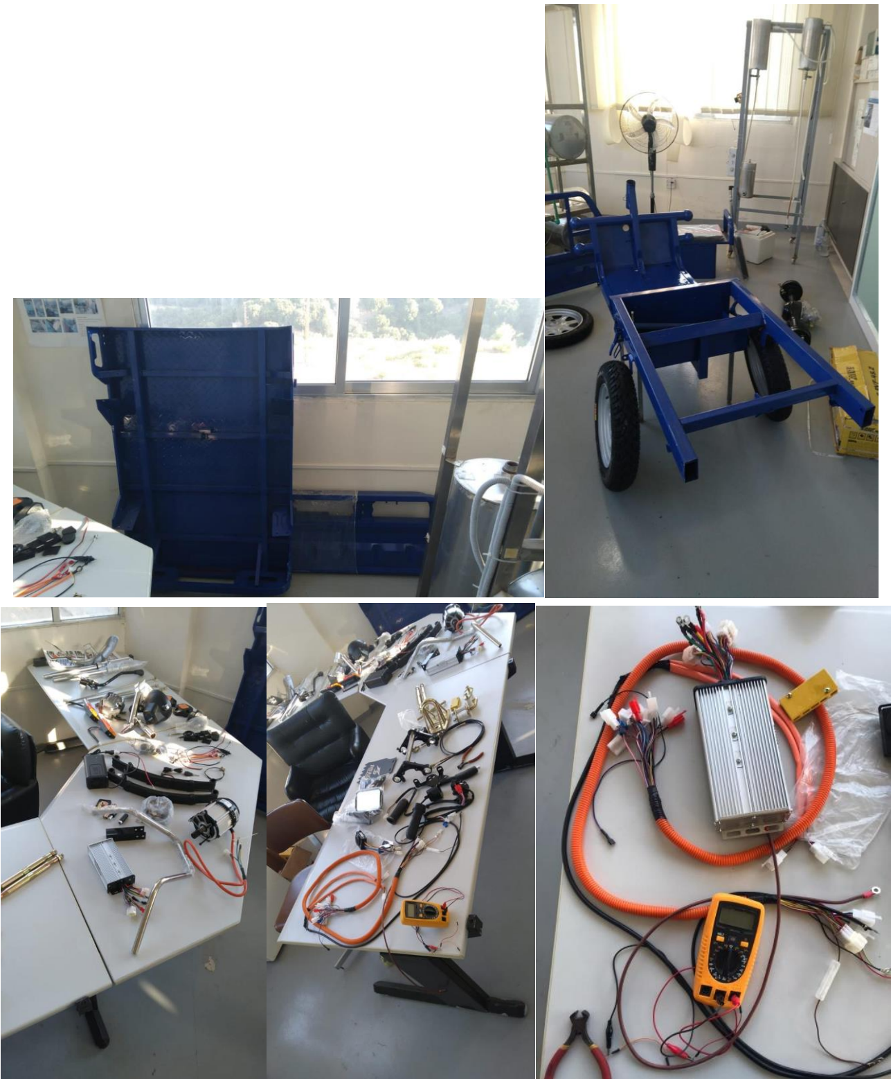
1000w controller and connecting wires
