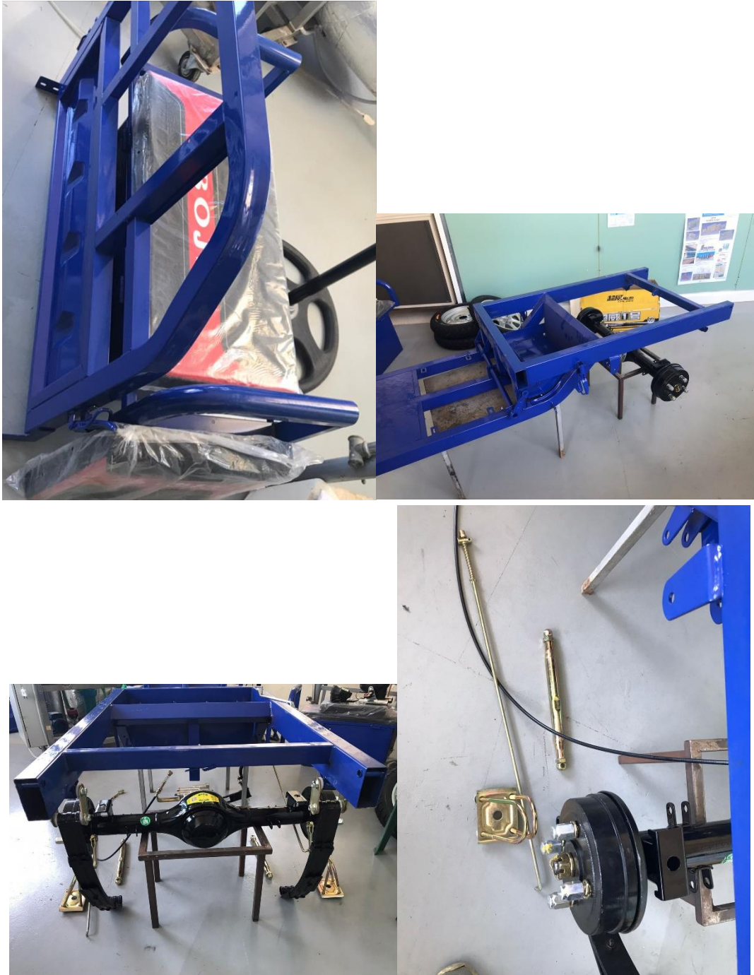
Rear suspension, shock absorber, and brake drum
