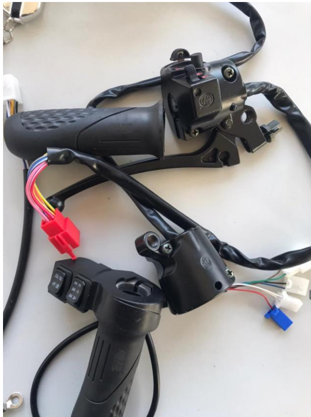
Throttle handelbar and speed controller
