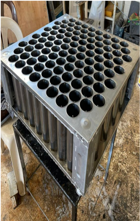
Here is how our cleaning of the Electro-Filter was done
