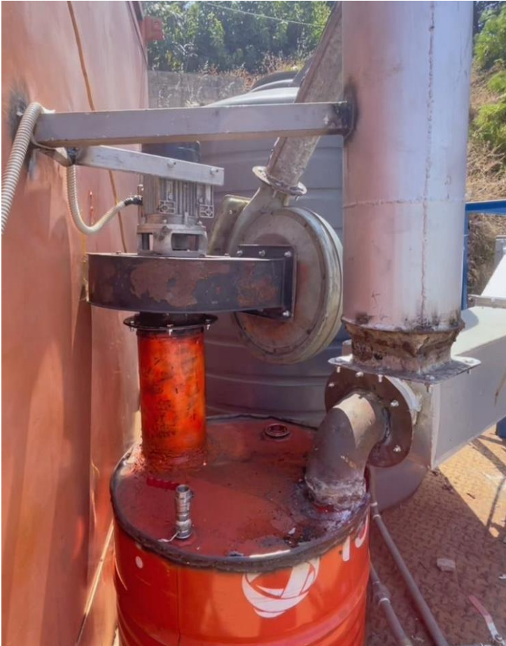
Flow gas into Barrel water Filter Test (24.6.2024)
