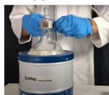
Reflux at 40-50 °C for 1-2h
