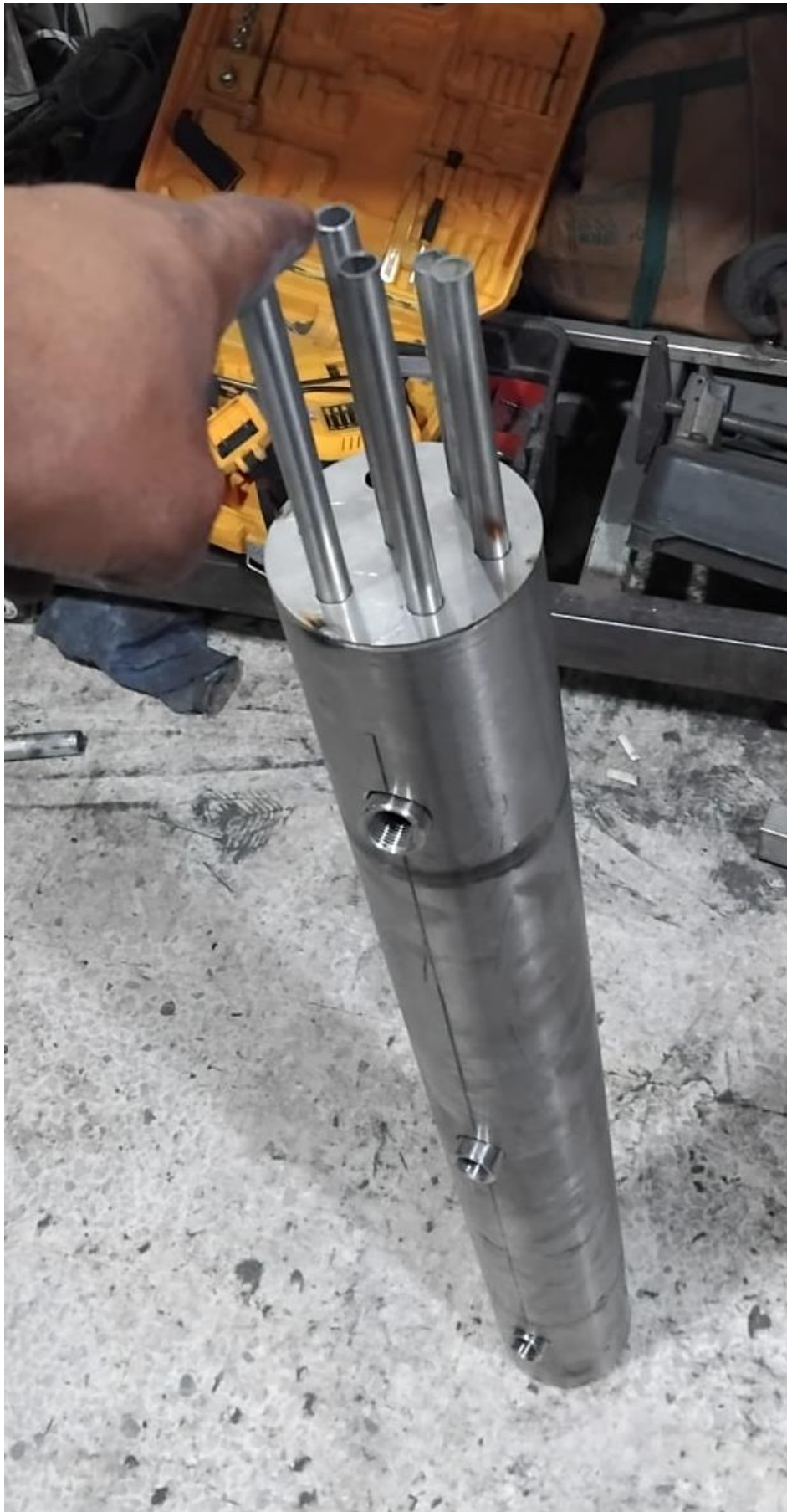
Whole condenser inlets tubes and jacket (view 2) 10.09.2024
