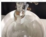
Cooling the reaction in the round bottom flask by an ice bath
