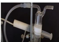
3. After the purification step the gas should go through the bubbler connected to collection tube.
