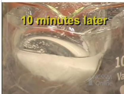
9. 10 minutes later, the aspirin should be precipitated.
