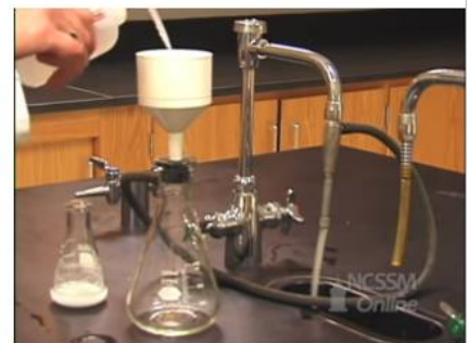
11. Add small amount of cold water on the filter paper.
