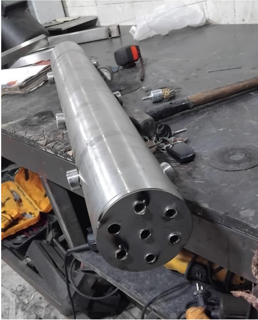
Whole condenser inlets tubes and jacket (view 3) 10.09.2024
