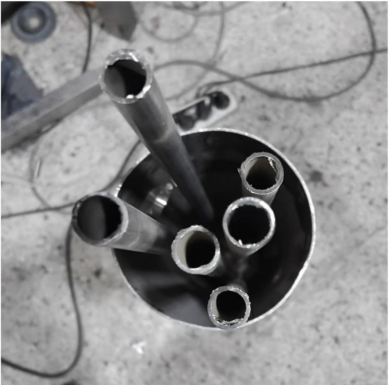
Whole condenser inlets tubes and jacket (view 1) 10.09.2024
