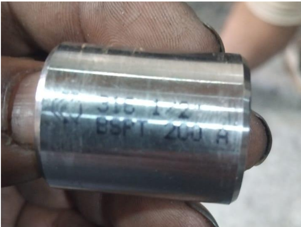
Stainless-steel 316 female connector (condenser inlet) 14.08.2024
