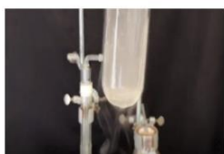
5. Sulfur dioxide is transformed to liquid form
