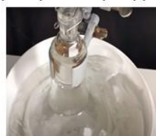
Cooling the reaction in the round bottom flask by an ice bath
