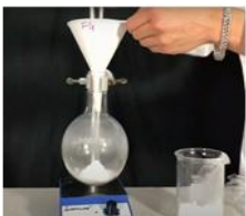
Add sodium acetate in the round bottom flask
