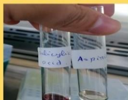
Results of qualitative test of FeCl 3 with salicylic acid (purple) and aspirin (transparent)
