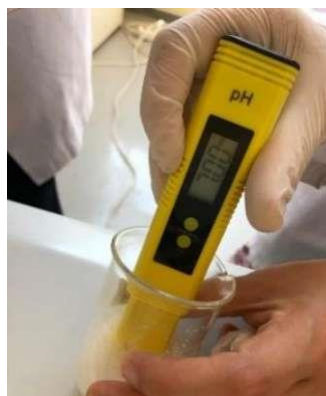
Figure 32: Adjustment of the pH of the reaction mixture to the value 7
