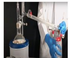
Distillation of acetic anhydride at 110 °C
