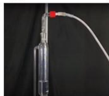
Put gas safety outlet
