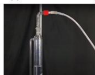
Put gas safety outlet
