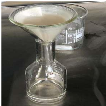
Figure 33: Filtration of the reaction mixture
