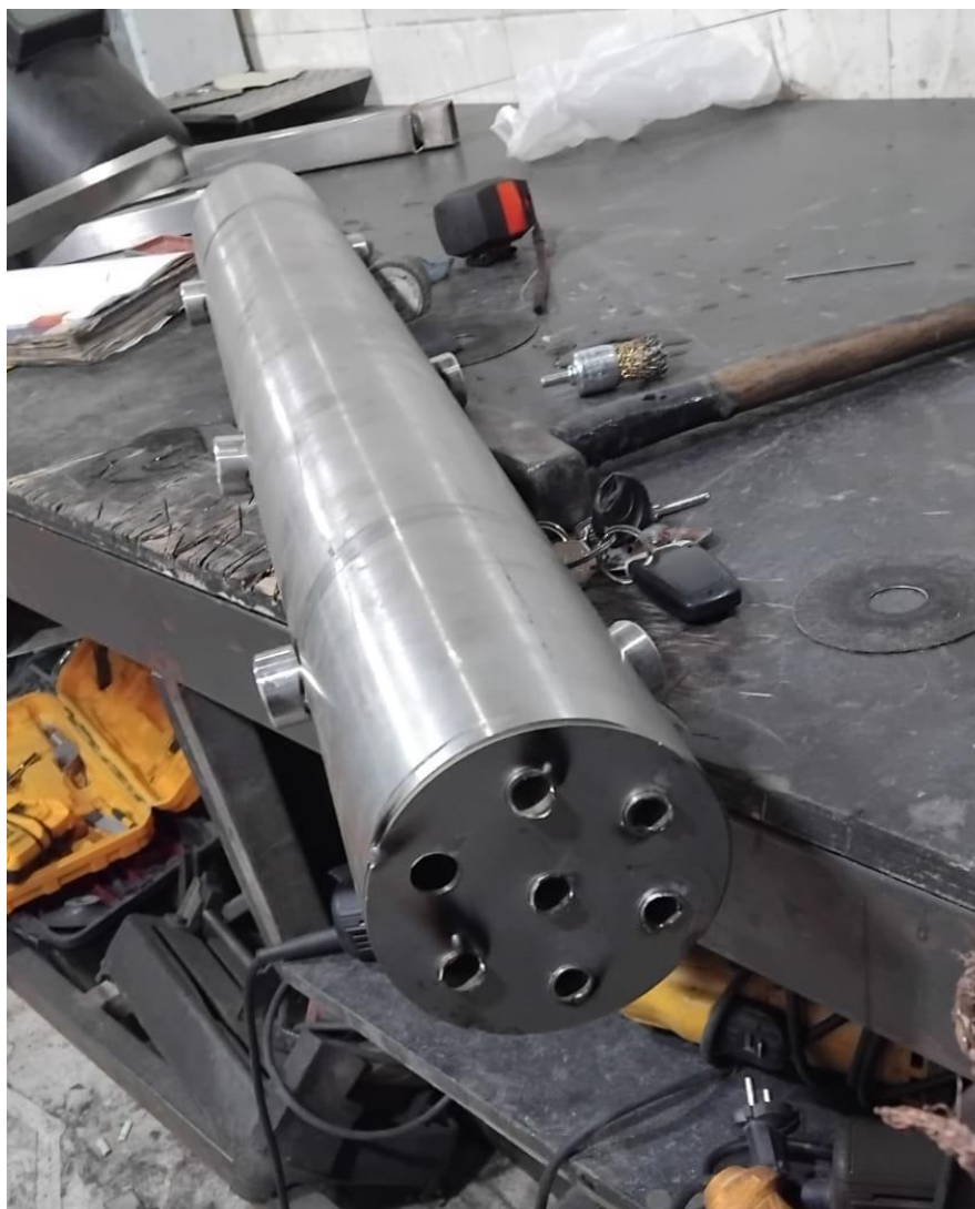
Whole condenser inlets tubes and jacket (view 3) 10.09.2024
