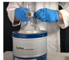
Reflux at 40-50 °C for 1-2h
