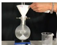
Add sodium acetate in the round bottom flask
