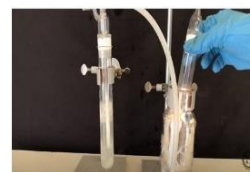
4. Put the collection tube in dry ice bath.
