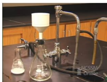
10. Now, we filtrate the aspirin by a vacuum filtration.
