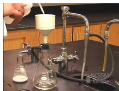
11. Add small amount of cold water on the filter paper.
