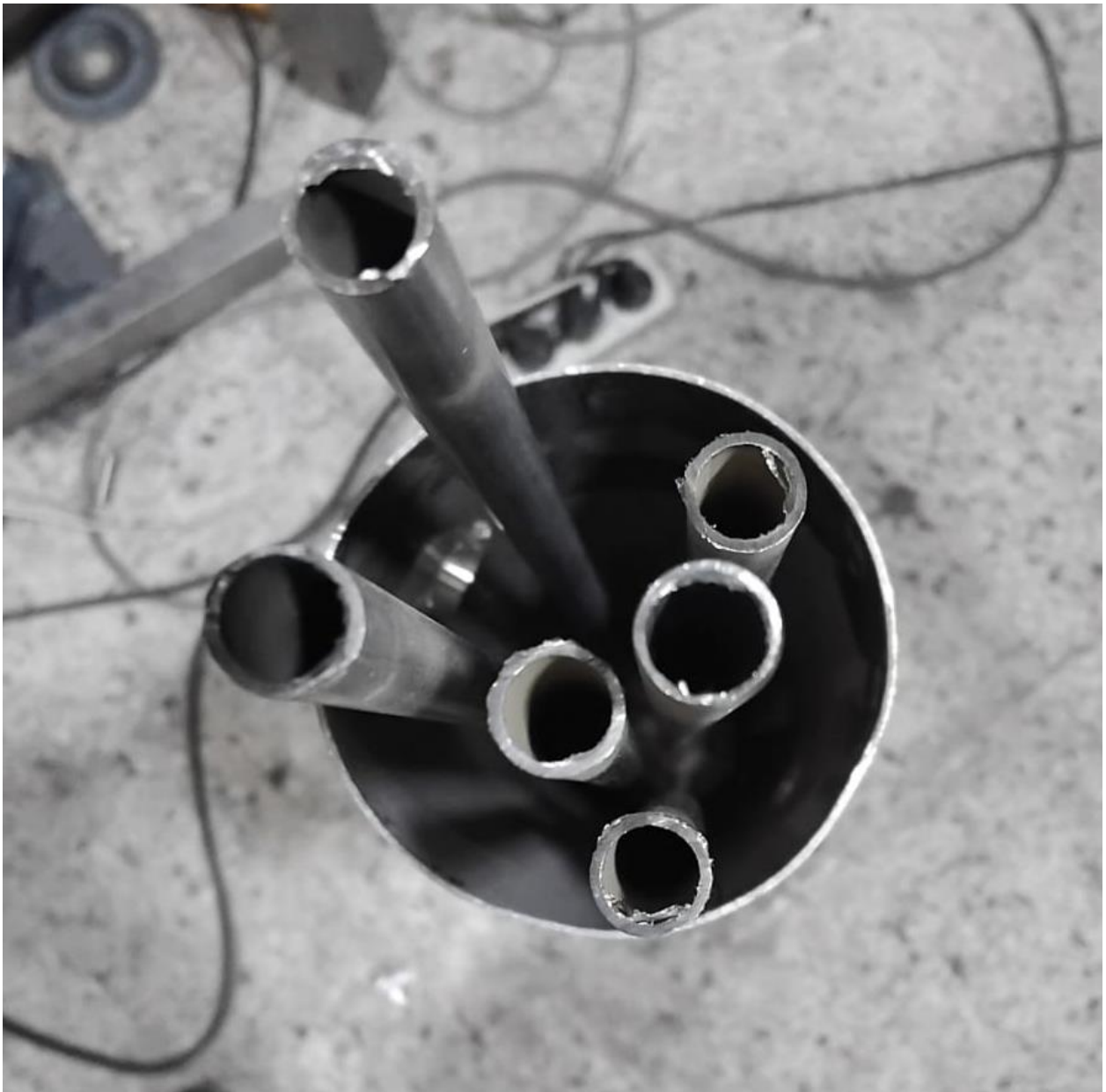
Whole condenser inlets tubes and jacket (view 1) 10.09.2024
