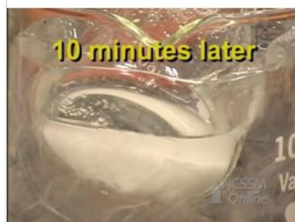
9. 10 minutes later, the aspirin should be precipitated.
