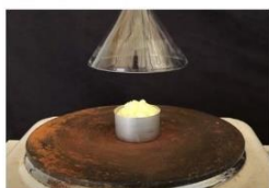
1. Burning the Sulfur powder in presence of \text{O}_2 with fire gun.
