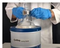
Reflux at 40-50 °C for 1-2h
