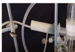
2. Filter the sulfur dioxide through a syringe contain cotton and calcium chloride \text{CaCl}_2 .
