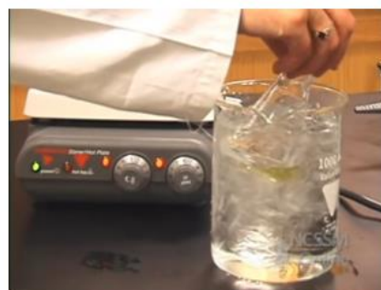
8. Put the volumetric flask in ice, so aspirin can start precipitating.
