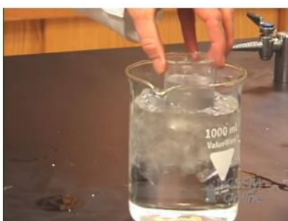
16. Put the beaker in ice to recrystallize.
