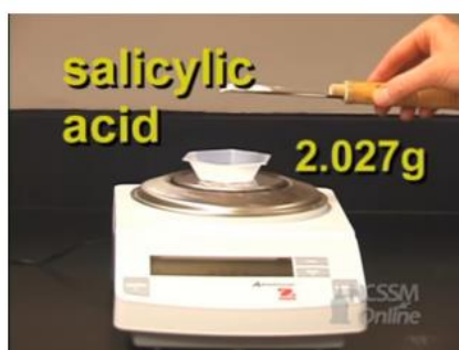
1. Weigh 2.027 g of Salicylic acid, then put then into a volumetric flask
