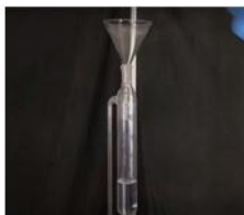
Add acetyl chloride using addition funnel
