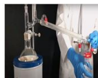
Distillation of acetic anhydride at 110 °C
