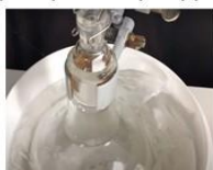
Cooling the reaction in the round bottom flask by an ice bath
