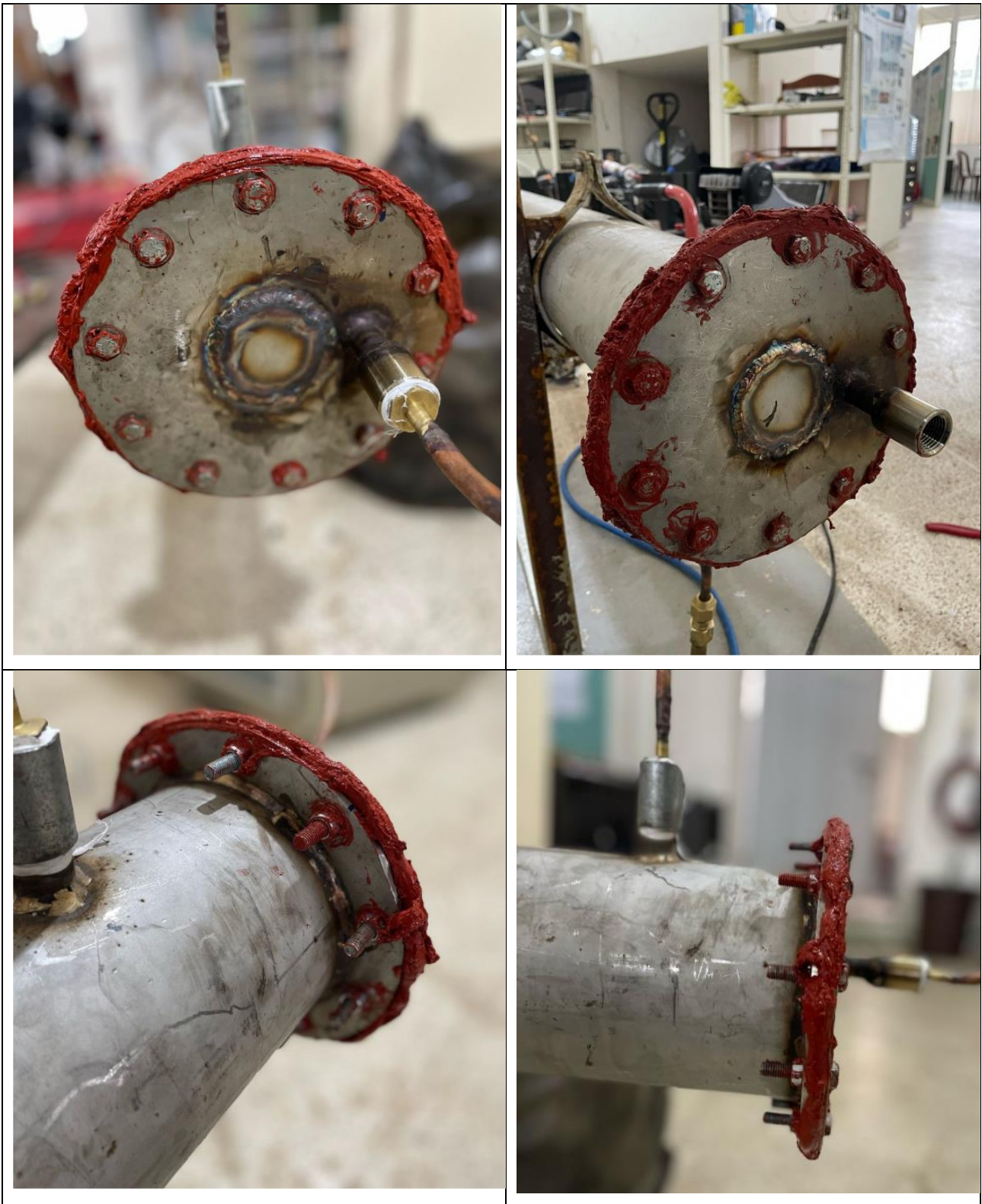
Also the 2 holes in the top and bottom were closed with stainless steel because the system was leaking in the middle of the pipe.
