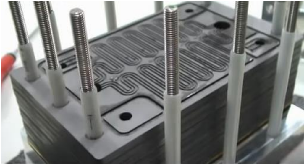
Fig. 75: First cell next to the current collector
