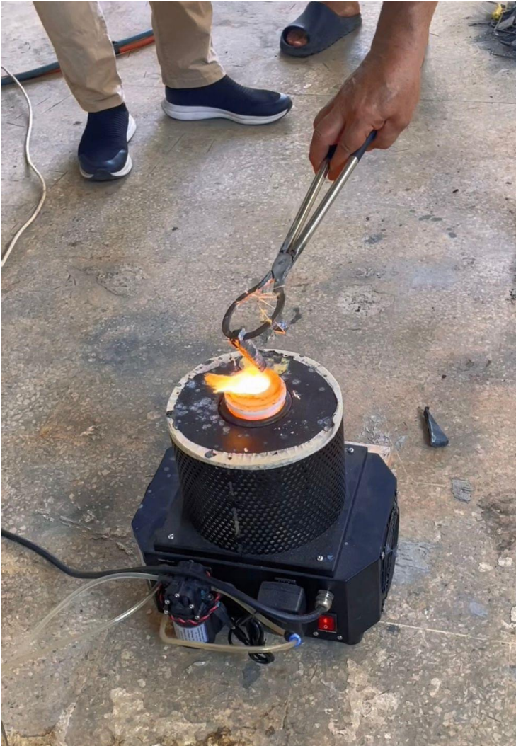
6. The problem occurred when we added too much iron into the pot, and the amount was more than necessary.
