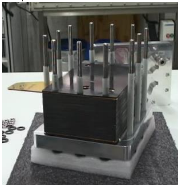
Fig. 73: Remove the end plate from the stack
