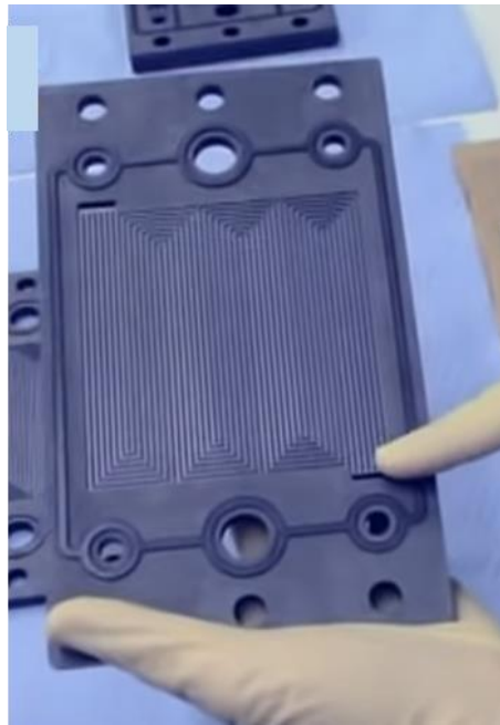
Fig. 78: Gas distribution channel with multiple support flow field, and field gasket at the front side
