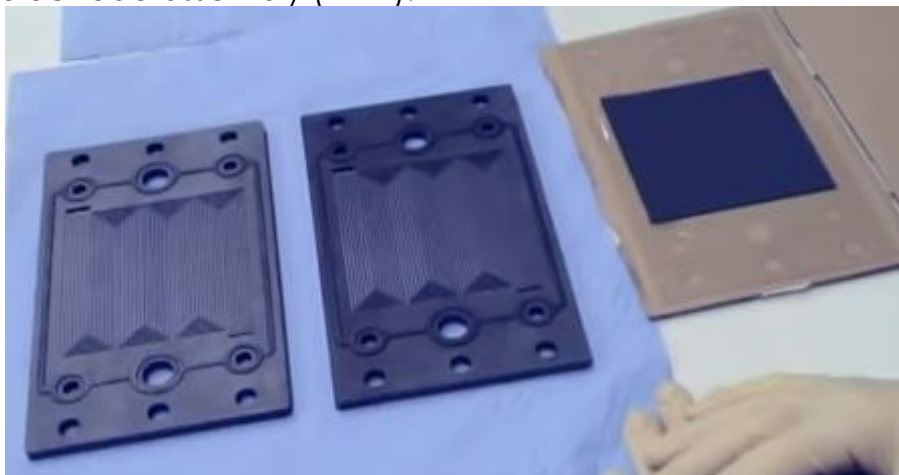
Fig. 76: Overview of a single cell (Two graphite plate and one MEA)
