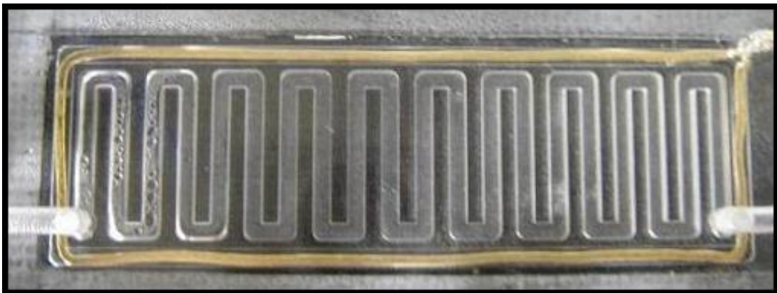
Fig. 67: Condensation of water produced by a PEMFC on the air channel wall. The gold wire around the cell ensures the collection of electric current
