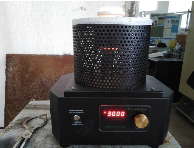
4. Heating stage 3: 5000 watts for 2 min
