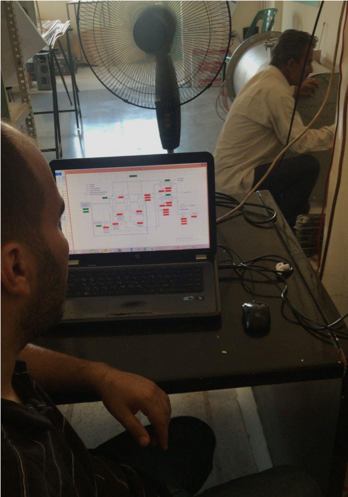
Turning on the system through the GUI after nitrogen purging for more than 10 minutes
