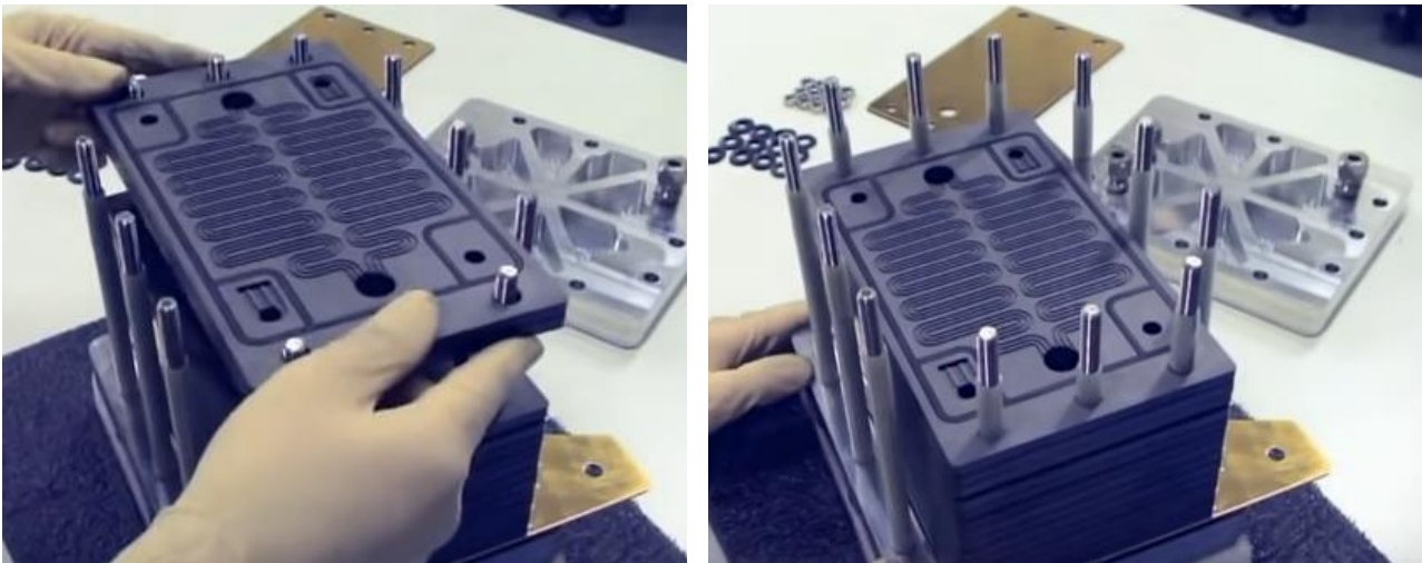
Fig. 86: Add the second cell
