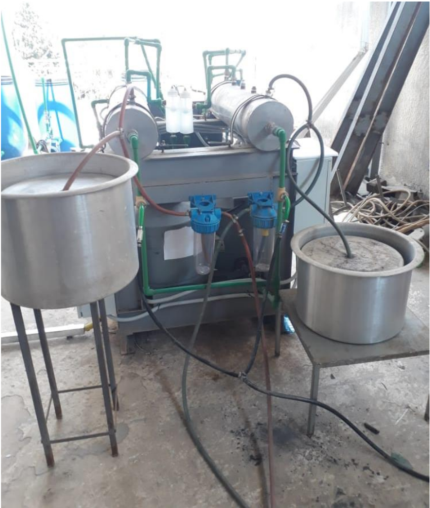
2) Pipe installation from O 2 and H 2 condenser to fuel burner with filters and expansion tanks
