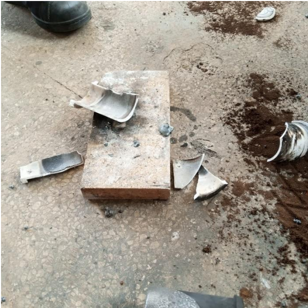
8. As a result, the clay pot exploded due to the pressure from the excessive expansion.
