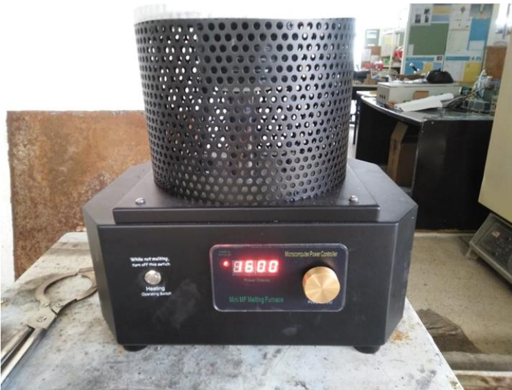
3. Heating stage 2: 3000 watts for 5 min
