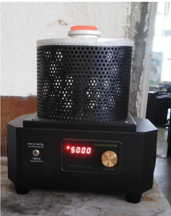
4. Heating stage 3: 5000 watts for 2 min
