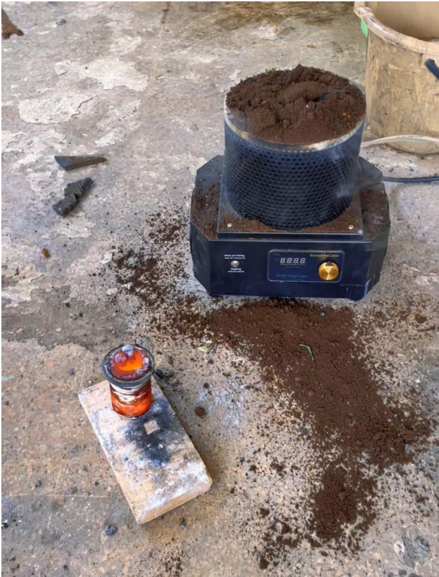
8. As a result, the clay pot exploded due to the pressure from the excessive expansion.
