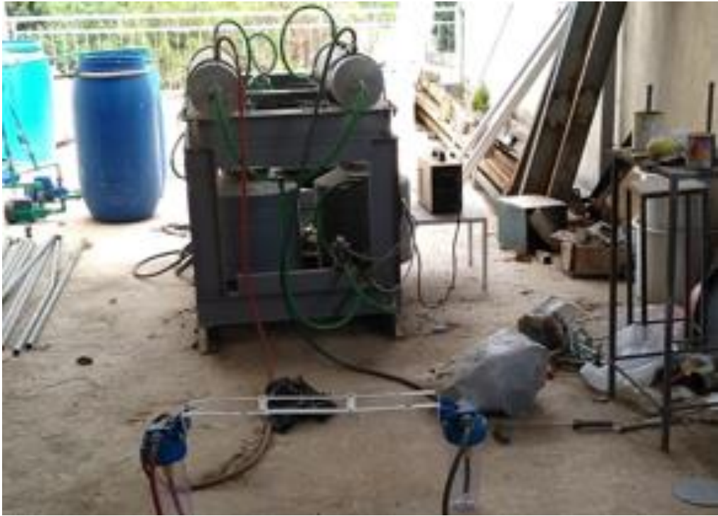
2) Pipe installation from O 2 and H 2 condenser to fuel burner with filters and expansion tanks
