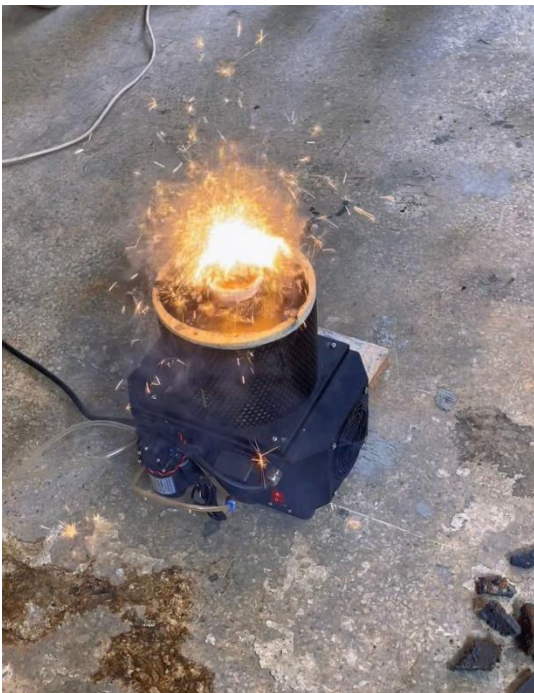
7. The iron expanded excessively due to this excess amount and resulting heat.
