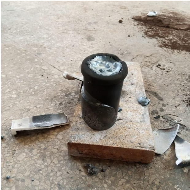
8. As a result, the clay pot exploded due to the pressure from the excessive expansion.
