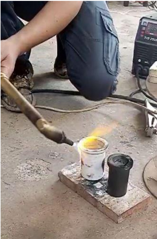
5. We placed the clay core pot and the lead pot with the Iron parts to melt them
