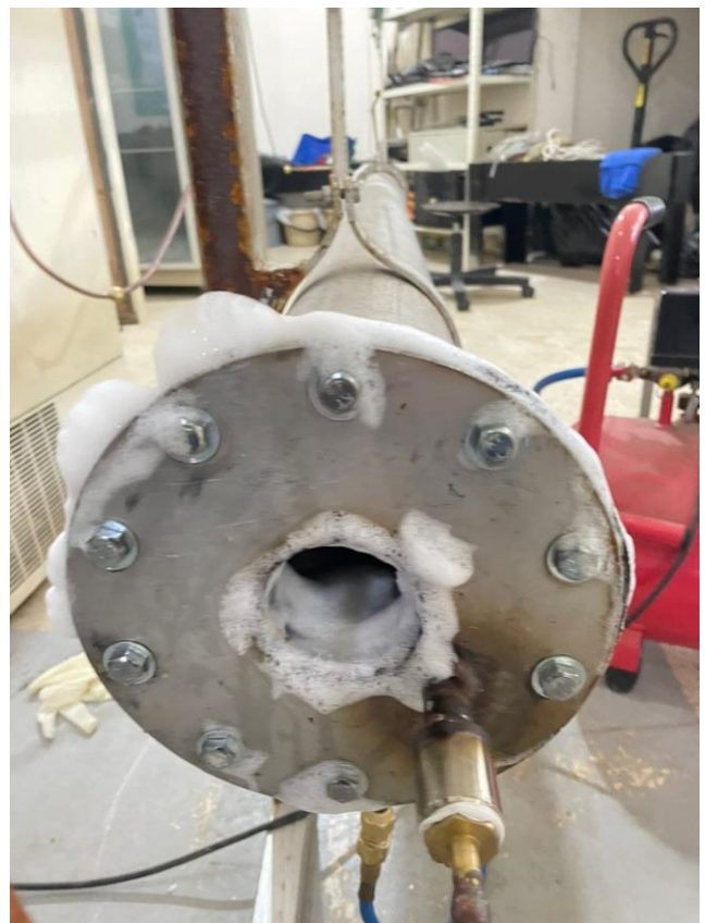
The leaking test started and unfortunately, the third type didn't work due to leakage
