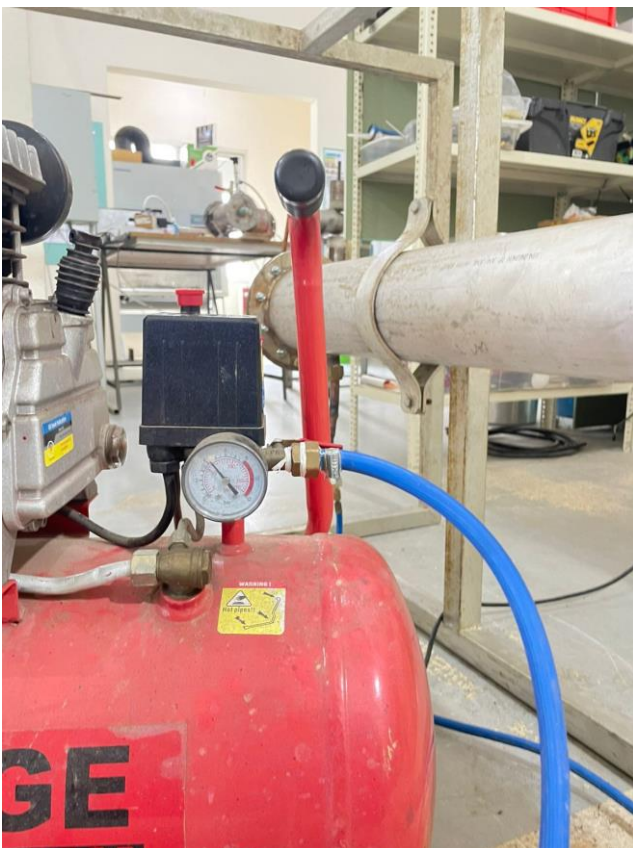
The leaking test started and unfortunately, the third type didn't work due to leakage
