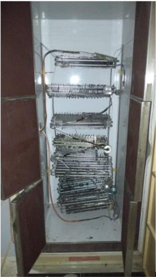
Figure 6. Cooler Tube Implementation
