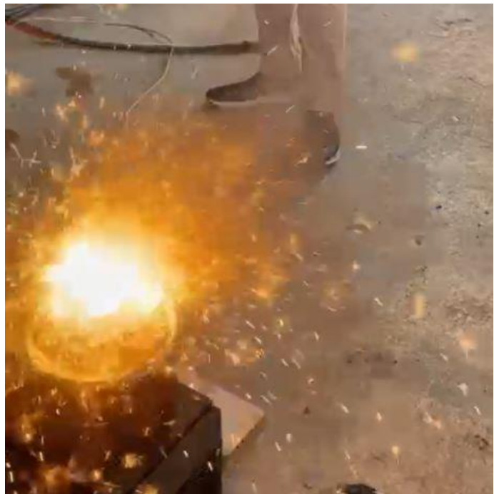
7. The iron expanded excessively due to this excess amount and resulting heat.
