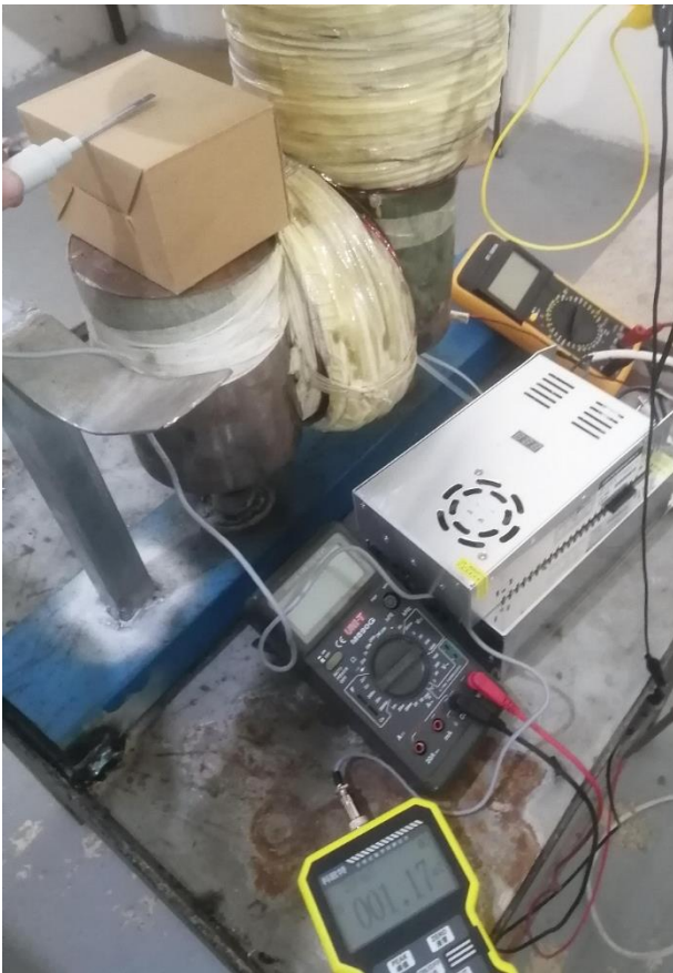
Figure 572: System is off and the teslameter displays a reading of 1 millitesla
