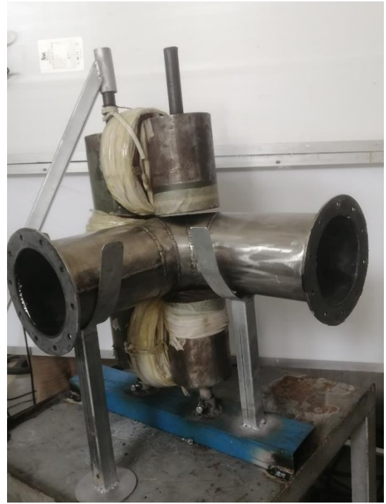
Figure 52.1: C-shaped electromagnet along the mass sector tube
