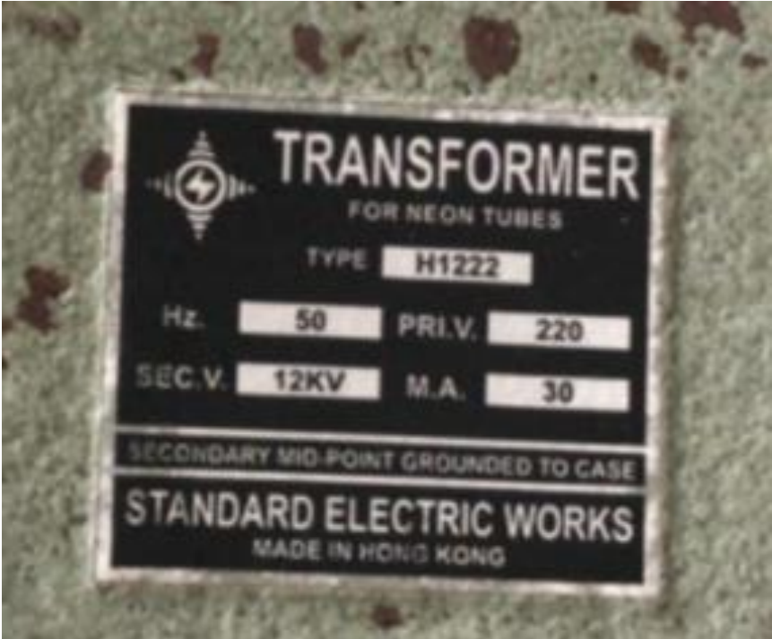
This transformer is an AC mode output, to convert to DC mode we use 4 diodes (30KV.0.5A)
