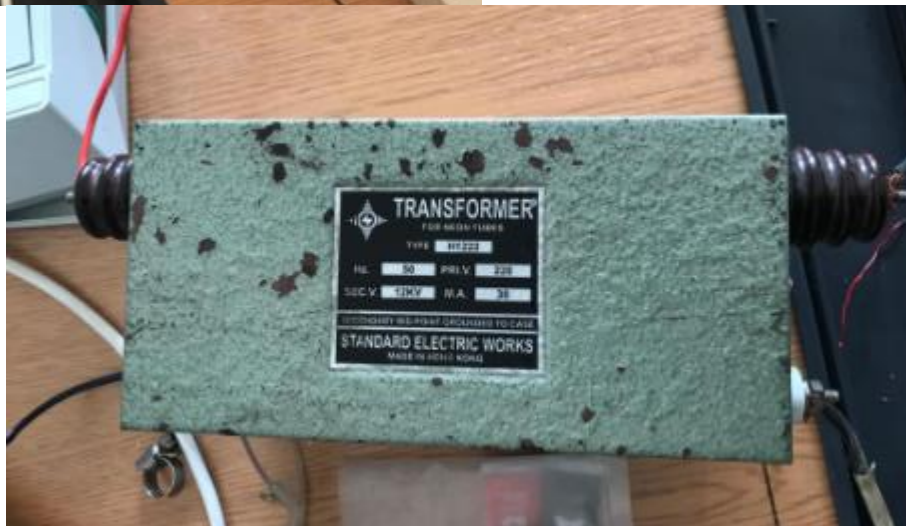
Transformer ( 12kv, 30 mA, 50hz)
