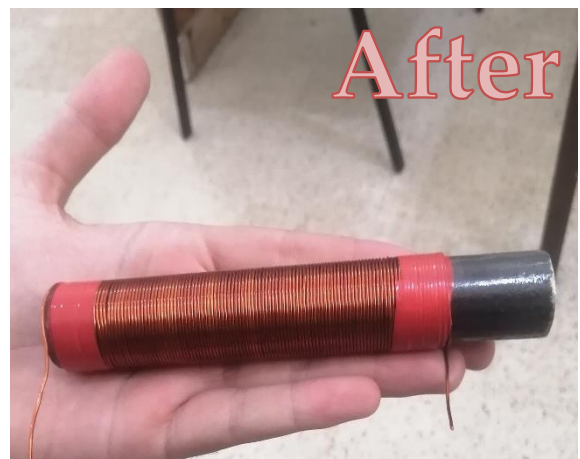
Figure 49: The small iron section with 5cm, before and after winding the copper
