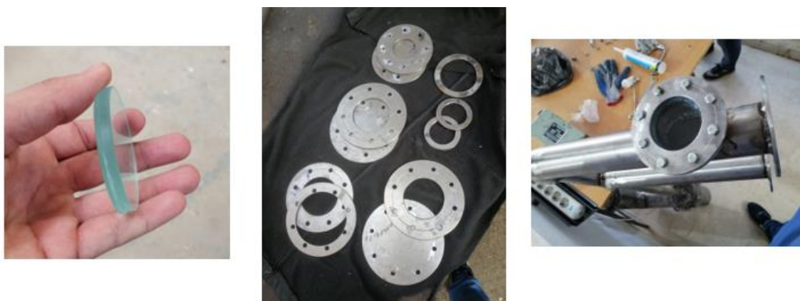
Figure II. 2: Preparing the window for X-rays with the appropriate flanges
