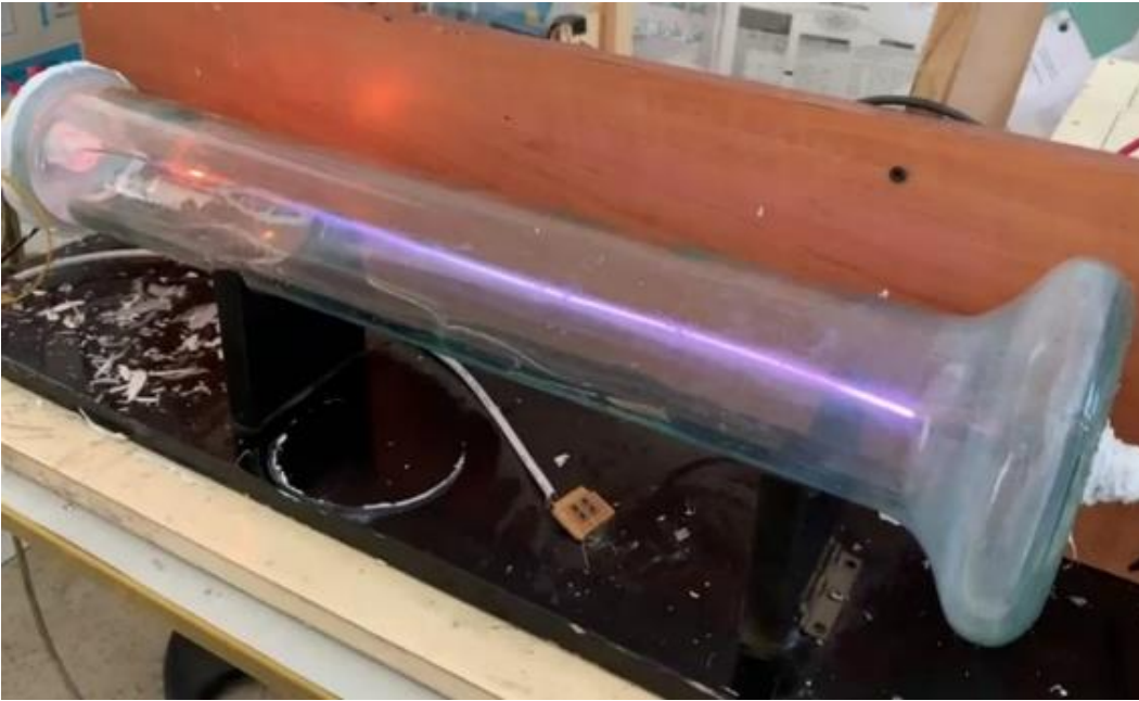
Figure III. 32: ignition of the tungsten lamp and appearance of the electron trajectory
