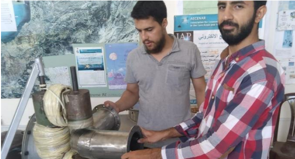
Figure 52.3: C-shaped electromagnet along the mass sector tube in the mass spectrometer
