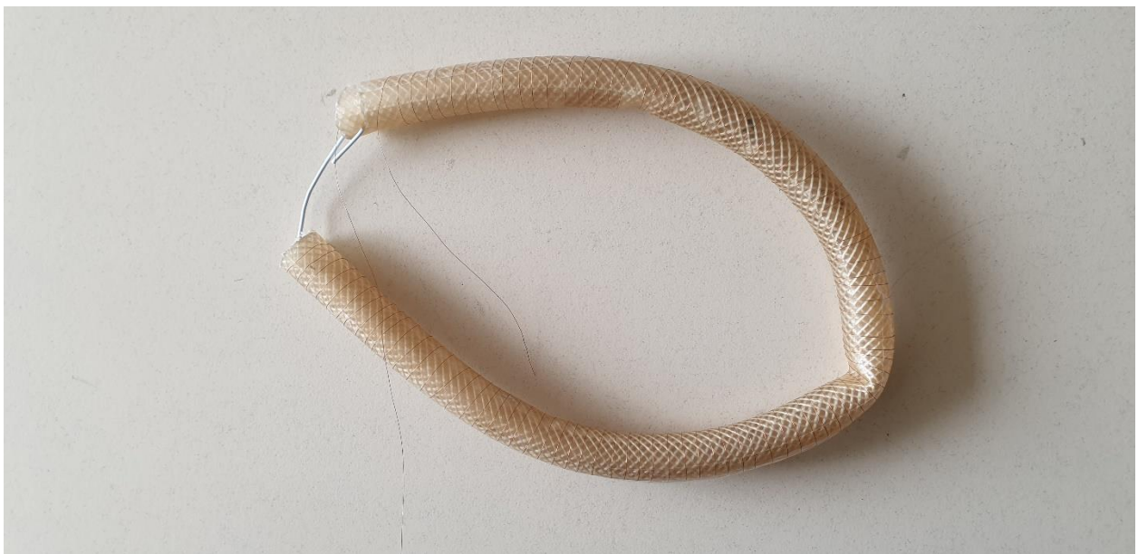
Fig.5: Rogowski Coil without integrator.
