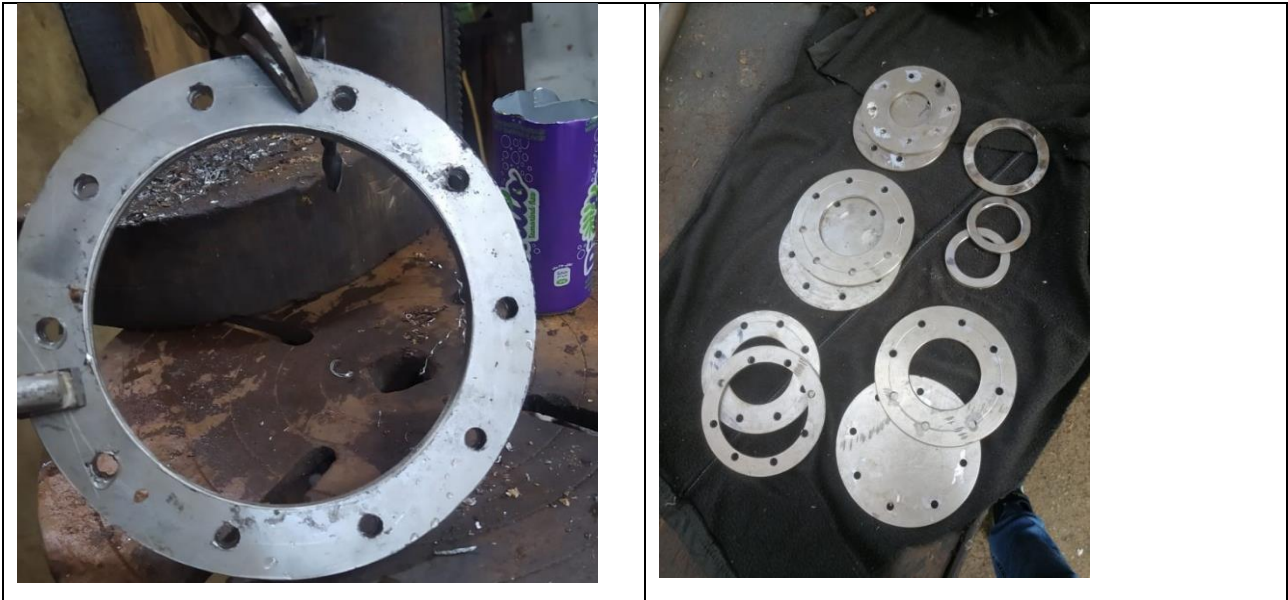
Figure II. 19: Fabrication of flanges for the various mass spectrometer components
