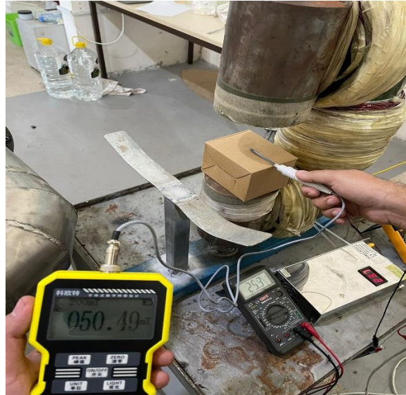
Figure 53: The teslameter displays a reading of 50 millitesla
