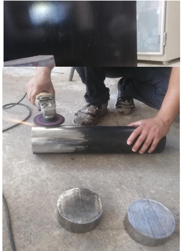
Figure 41: Polishing the iron from the black impurities from smaller to larger parts
