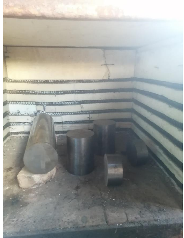
Figure 35: The iron bars inside the furnace
