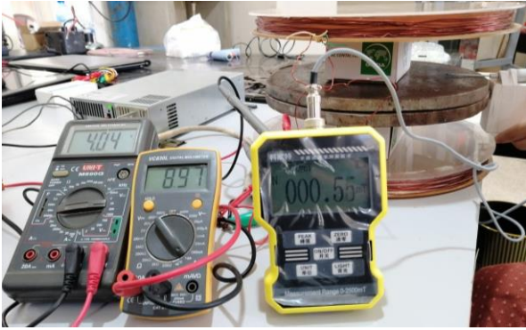
Figure III. 50: Evaluation of the magnetic field when inserting two ordinary iron plates in the center of the Helmholtz coil
