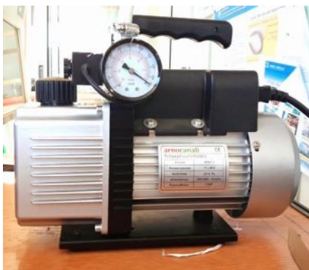
Figure I. 5 : Arnocanali Bistadium high pressure pump 421/H
