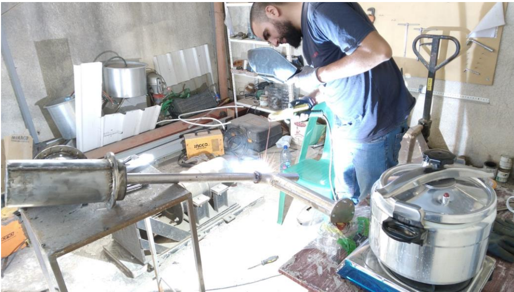
Figure II. 34: Welding during mass spectrometer manufacturing
