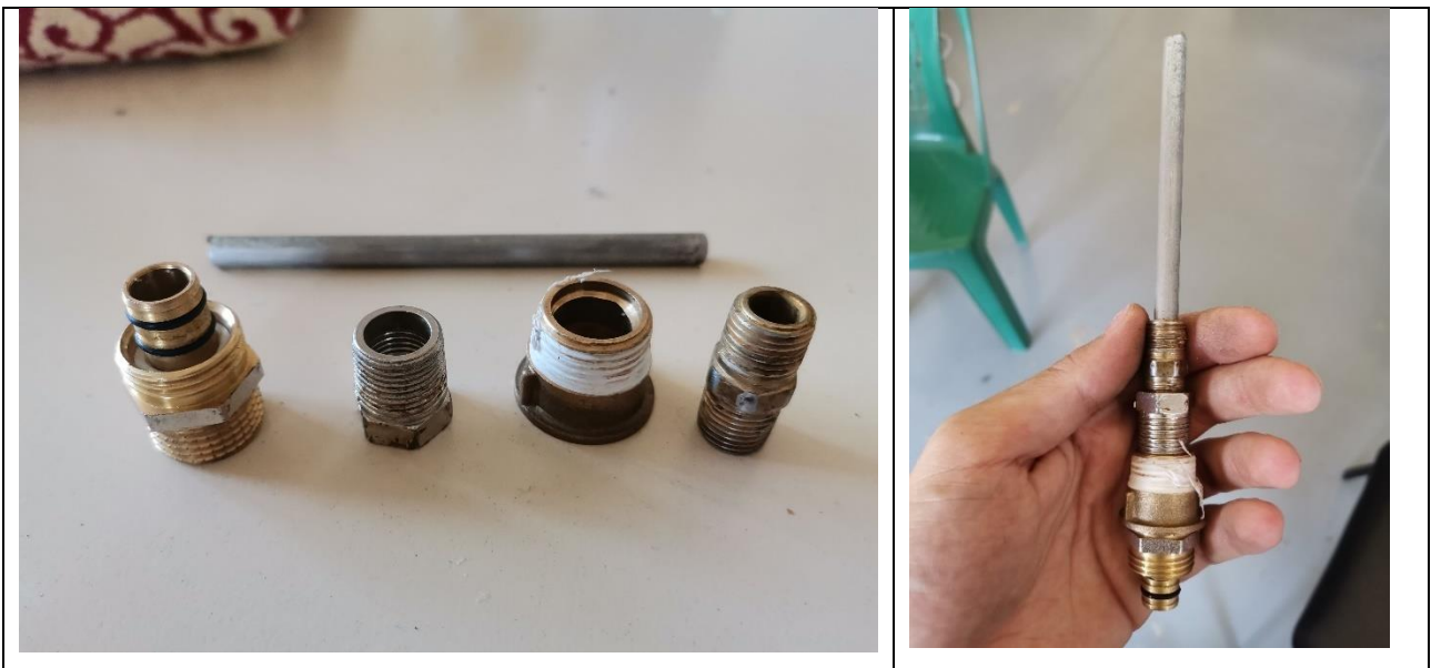
Figure 30: Cooper rod used as anode.
