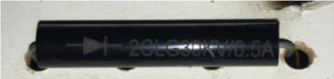
This transformer is an AC mode output, to convert to DC mode we use 4 diodes (30KV.0.5A)
