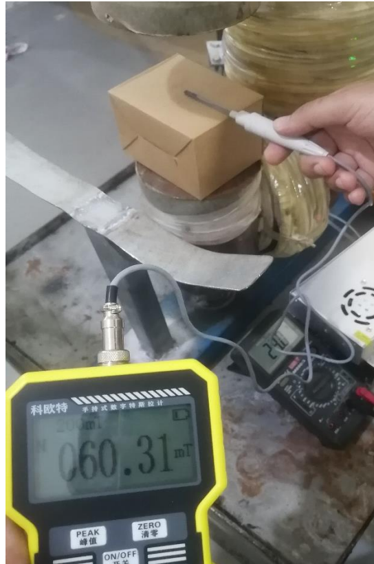
Figure 55: The teslameter displays a reading of 60 millitesla
