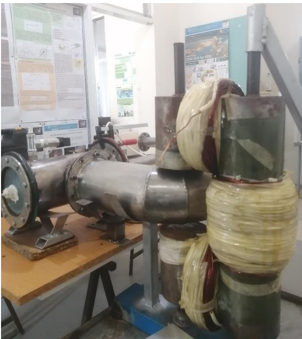
Figure 52.2: Fitting the mass sector tube in the air gap
