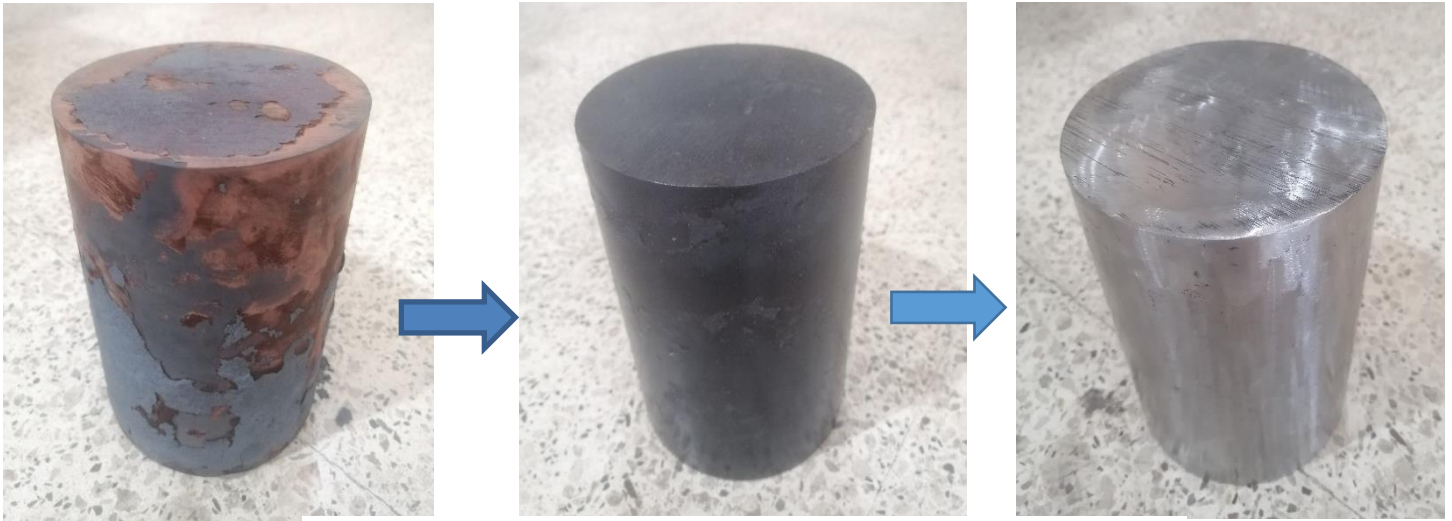
Figure 42: The difference steps of cleaning the heated iron
