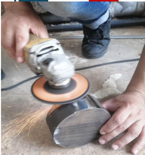
Figure 41: Polishing the iron from the black impurities from smaller to larger parts
