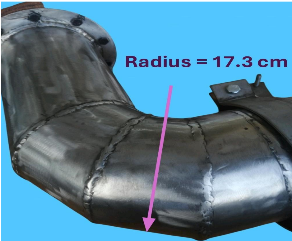
Figure 9: The maximum radius in the deflection zone for the mass spectrometer
