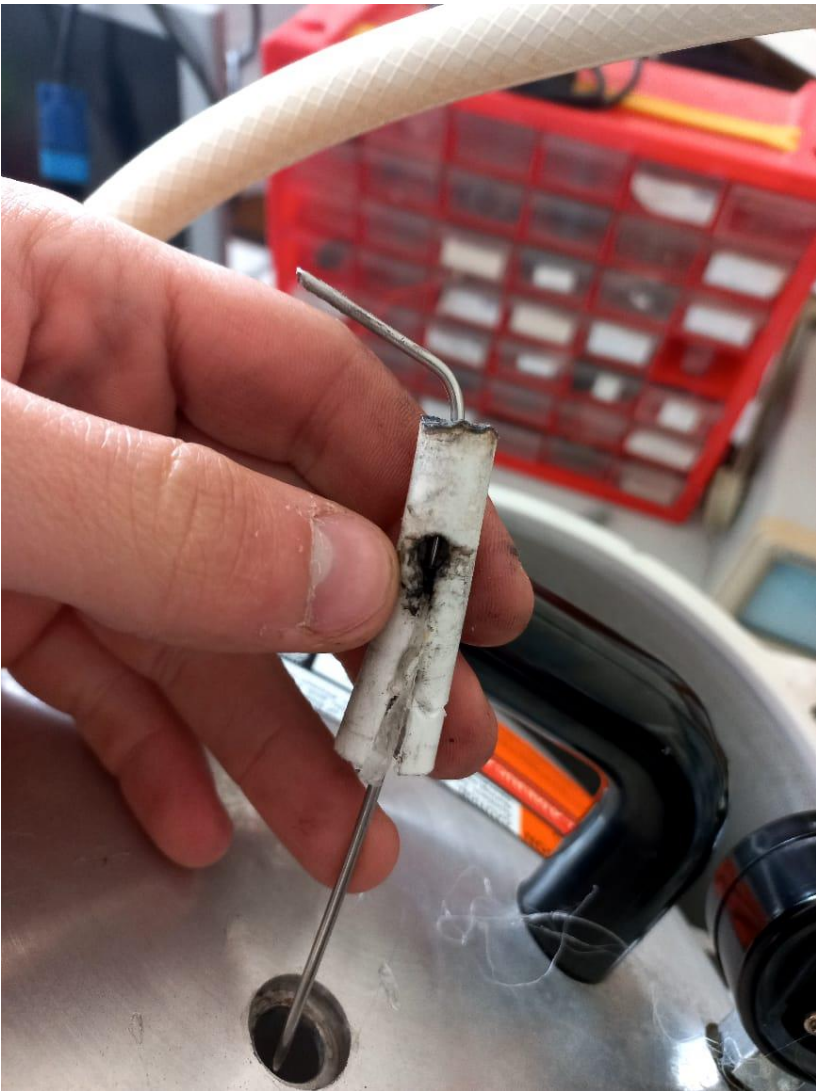
The electric spark milts the TEFLON.
