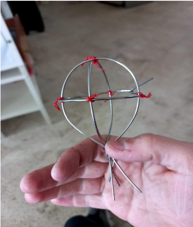
The cathode is a 7 cm diameter grid and consists of three 7 cm diameter rings that have been welded together, each ring is arranged such that the three rings form a spherical grid.
