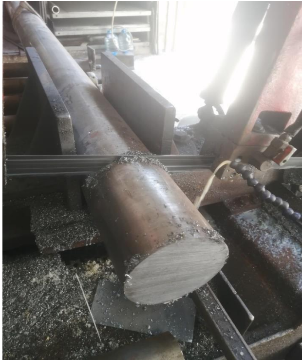
Figure 34: The cutting process for the iron
