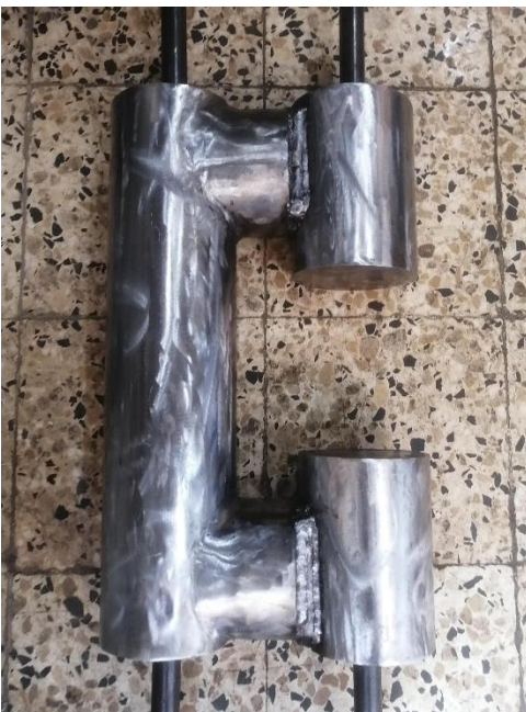
Figure 45: C-shaped iron core and its 2D ch
