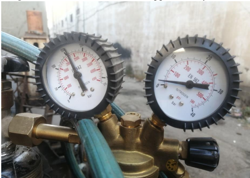
Figure 37: The nitrogen bottle filled with 150 bar
