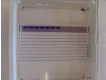
Fig.1.12: Agarose gel with samples loaded in the slots, before the electrophoresis process
