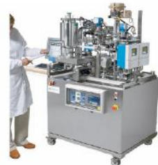
Fig. 1. Uniflux 10 system configured for cassette filters and holder.
