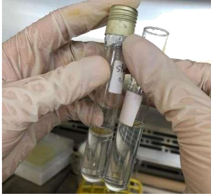
Figure 23: Comparison of turbidity between the bacterial suspension tube (right) and the standard McFarland tube (left).
