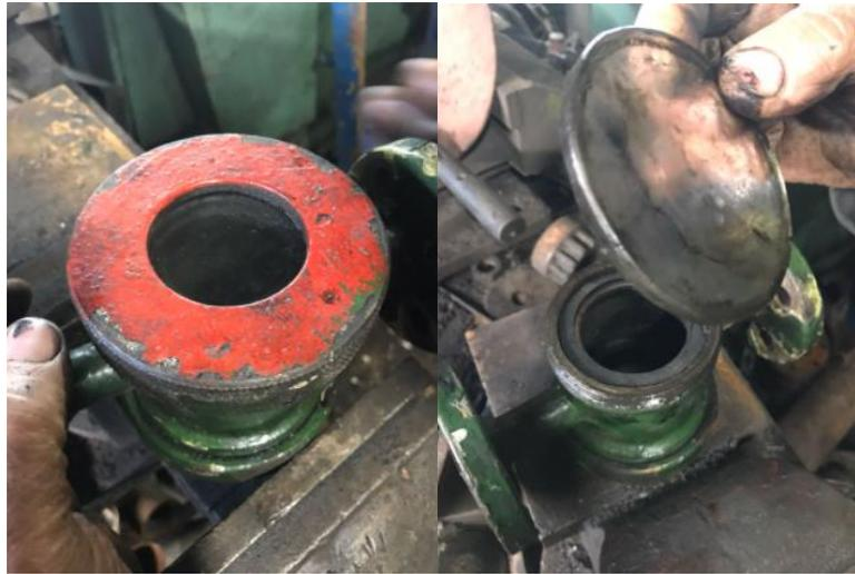
We will weld a Glass support on the Chamber.
