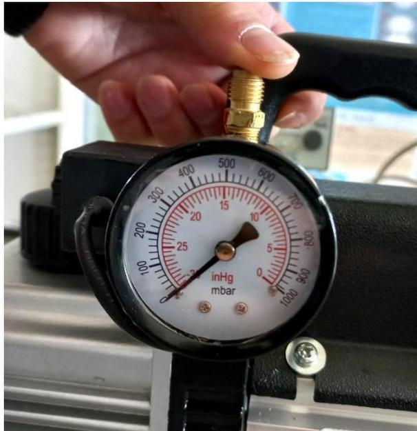
In order to be sure that the pump can reach its maximum, a thumb was putted where the pump is connected to the chamber.
