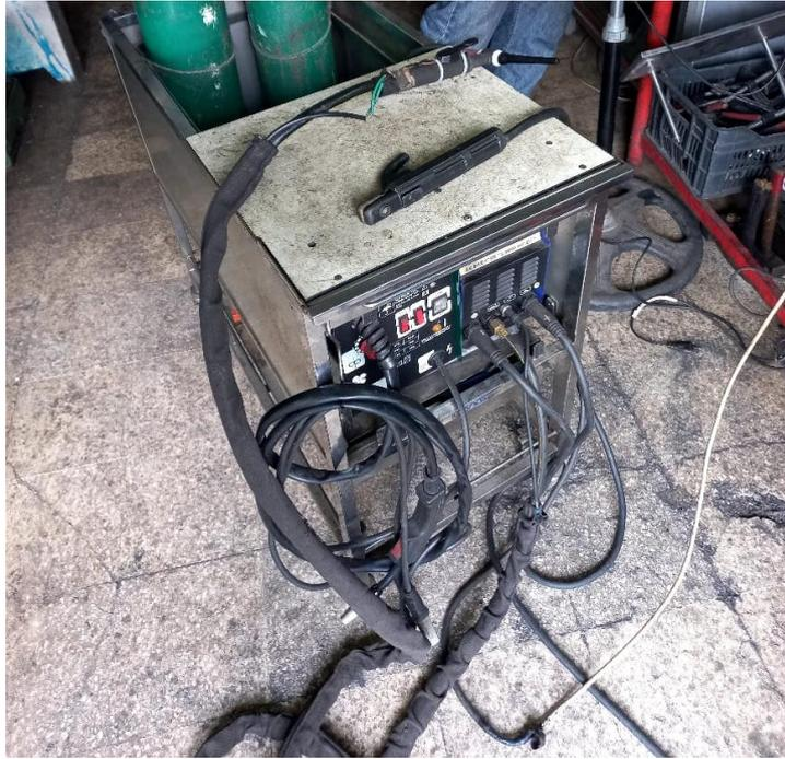
Figure 4-25. argon soldering electrical machine
