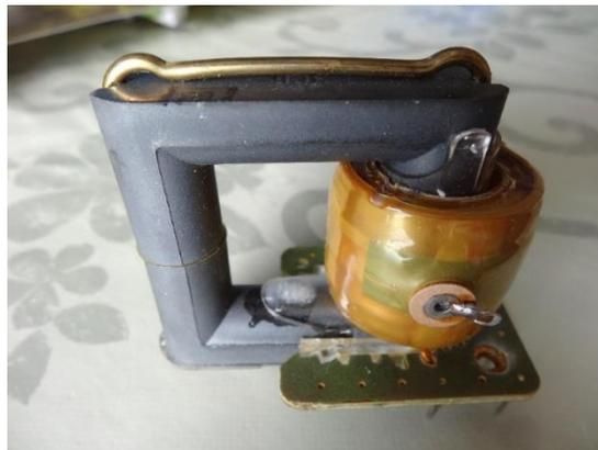
This combination delivers an output voltage of around 27 kV peak to peak at an input voltage of 24V using 4x4 windings on the primary side of the flyback transformer.
