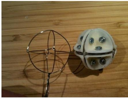
This particular jig is suitable for winding a grid with a diameter of 1.5" or 38 mm. It requires two 14" or 360 mm lengths of wire (tungsten or tantalum). The crossing intersections can be spot welded for a better rigidity.
