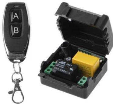
Figure 4-43. Wireless Remote-Control Receiver
