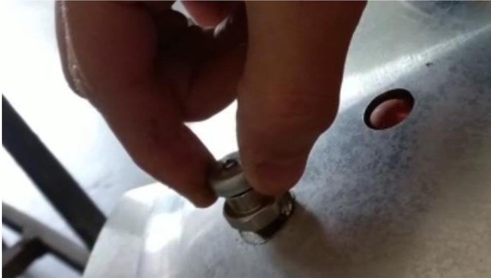
Figure 7-5 safety valve opened
