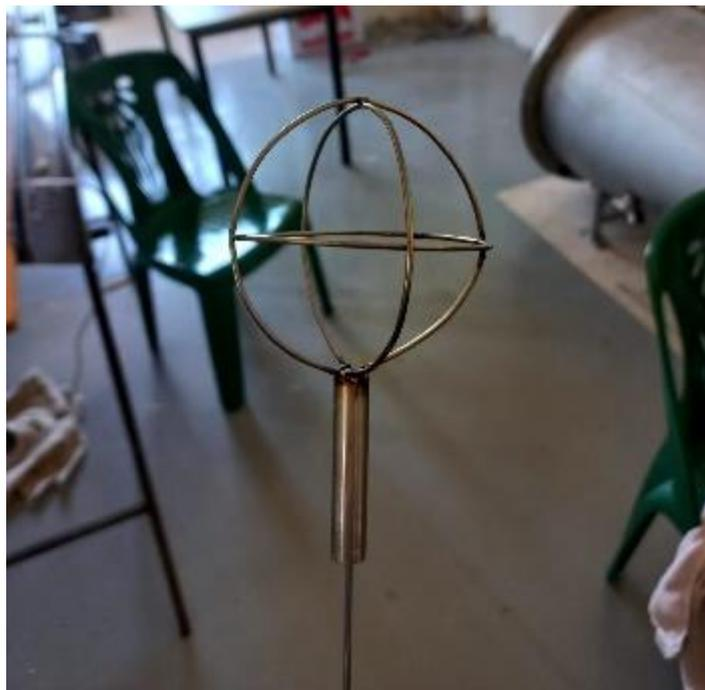
Figure 8-10. final form of stainless inner grid
