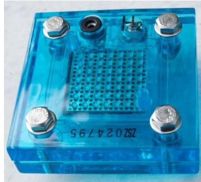
For those who want to construct their own PEM cell, the membrane is available at a price of approx. 16 EUR for a square piece of 10 cm<sup>2</sup> (sides of 3.3.cm). The power requirements are 1 A per cm<sup>2</sup> at 0.6V. The reason for constructing a PEM cell might be for producing Deuterium at high pressure or at a higher capacity by stacking cells. In that case the housing(s) of the cell(s) must be made of SS (stainless steel or inox or rostfrei) steel.
