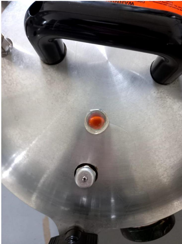
The air leakage was decreased 80 percent, where the pressure gauge shows that vacuum pump extracted 900 mBar from chamber.
