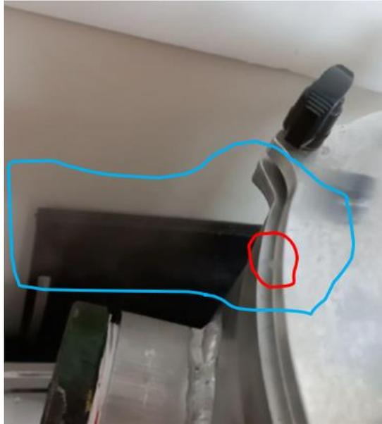
Figure 7-3. steam leakage
