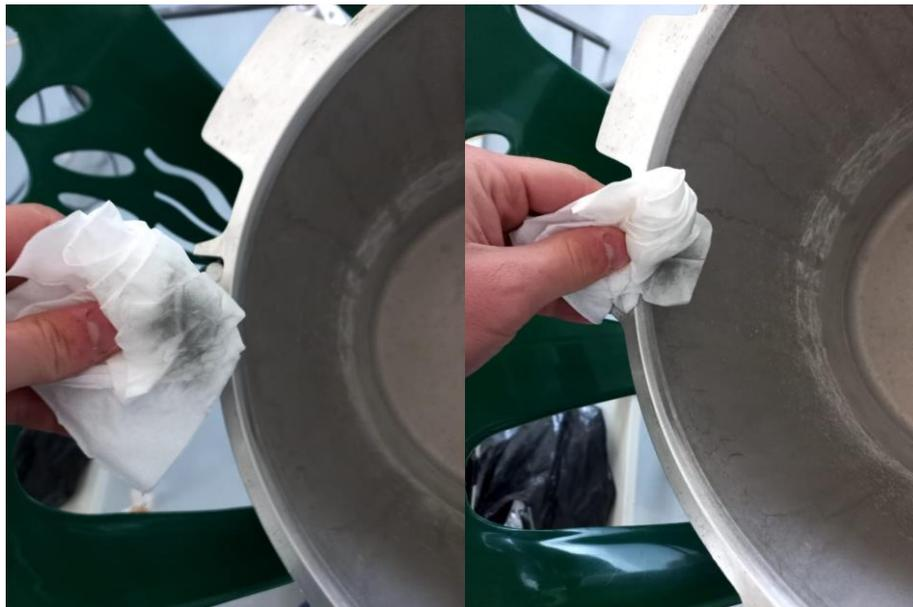
Figure 7-9. chamber edges lubrication
