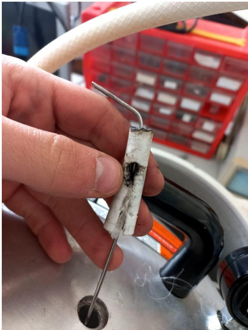
**The electric spark melts the TEFLON.**
