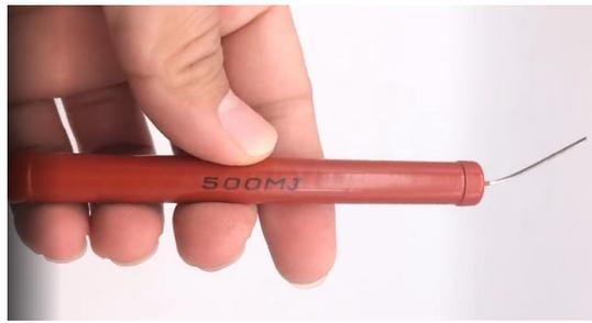
Figure 4-38. high voltage resistor of 500Mj
