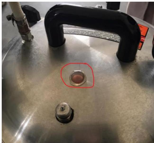
To stop air leaking we put silicon on the red circle, and we vacuumed the chamber
