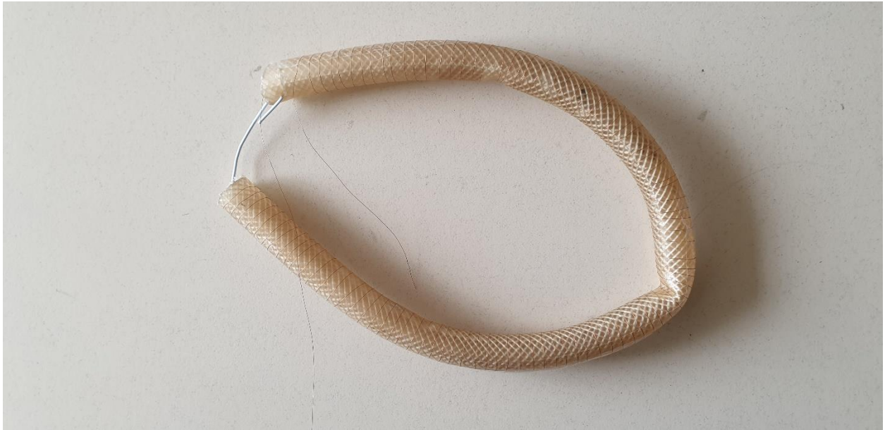
Fig.5: Rogowski Coil without integrator.
