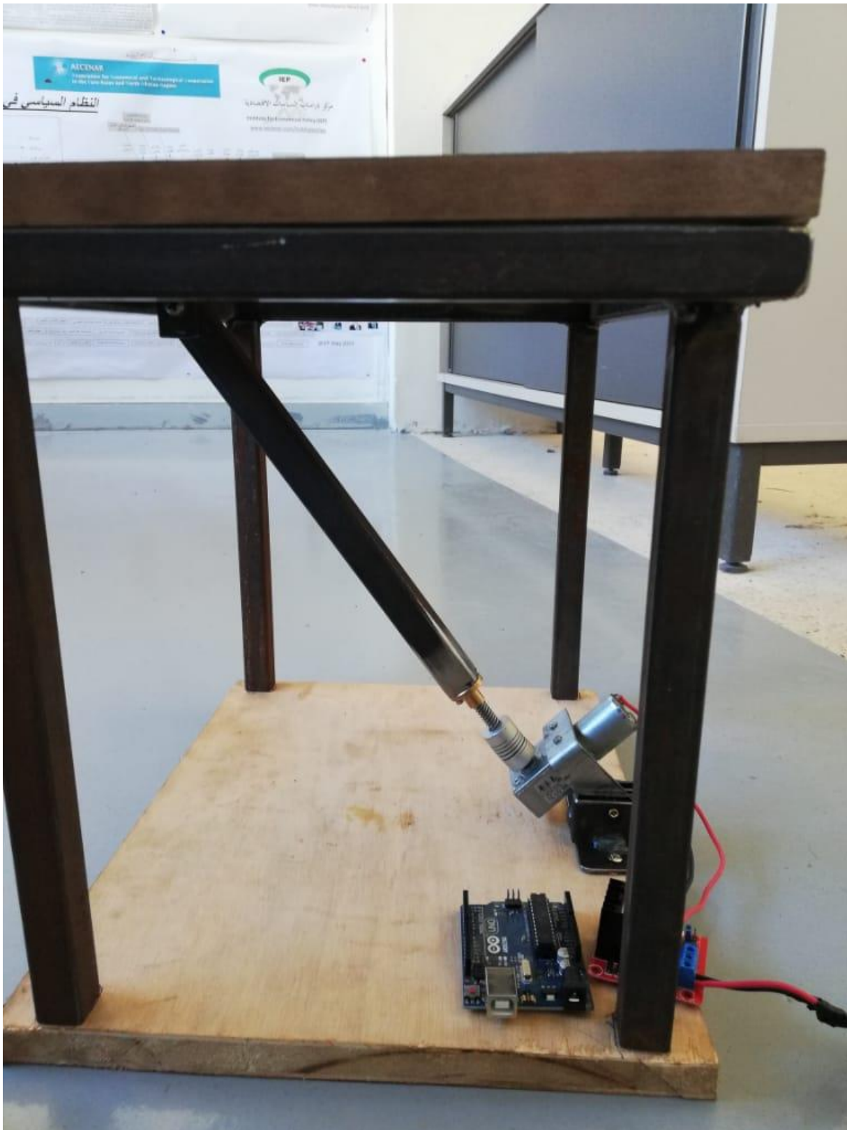
Figure 12: Mechanism that moves the Panel
