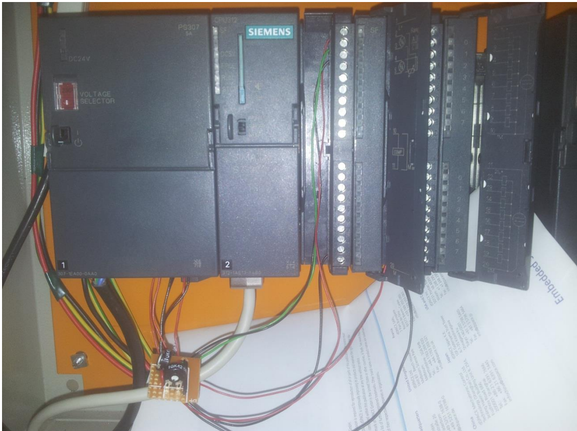
Figure 4.13: PLC Analog input connection
