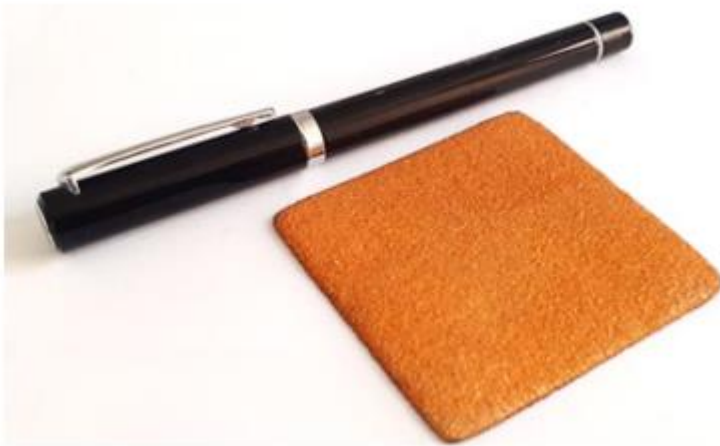
Figure 8. Fabricated three-layer radiation shield sample.
