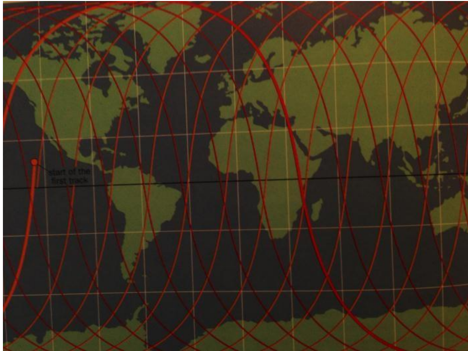
Figure 4.5: All rotations of the satellite around the earth during the day
