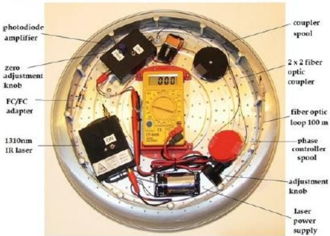
Figure 4: Assembled Sagnac interferometer
