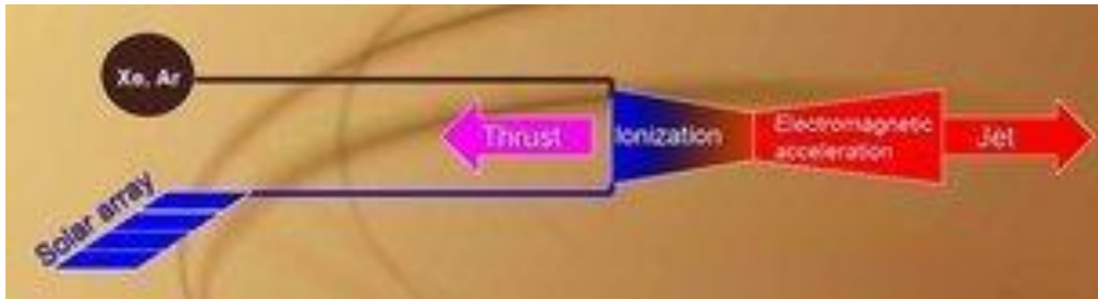
Figure 3.14: Hall Effect propulsion
